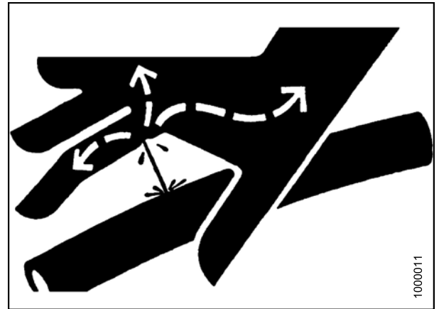
Figure 5.199: Hydraulic Pressure Hazard
