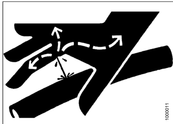
Figure 5.182: Hydraulic Pressure Hazard
