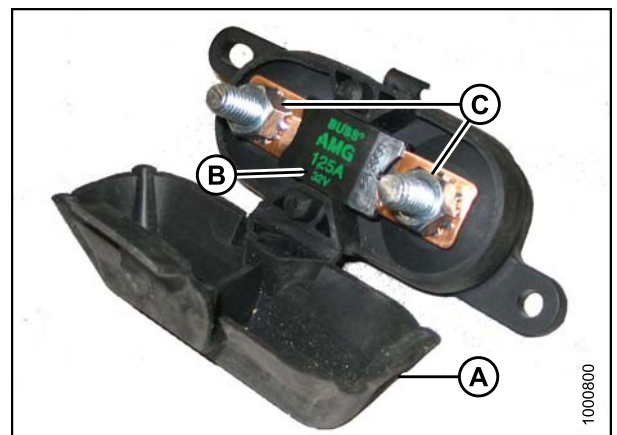
Figure 5.180: 125A Main Fuse
