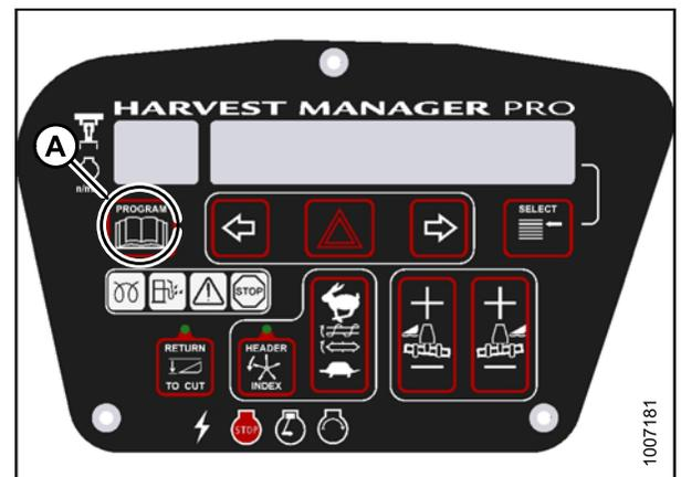
Figure 4.111: Cab Display Module (CDM)
