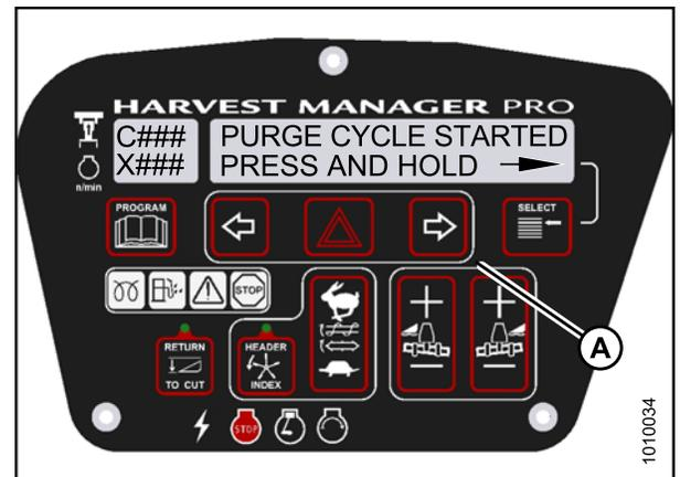
Figure 4.235: Hydraulic Purge Cycle
