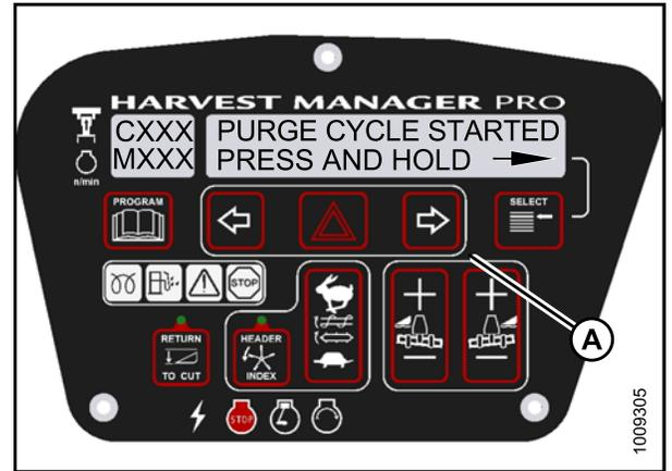
Figure 4.234: Hydraulic Purge Cycle
