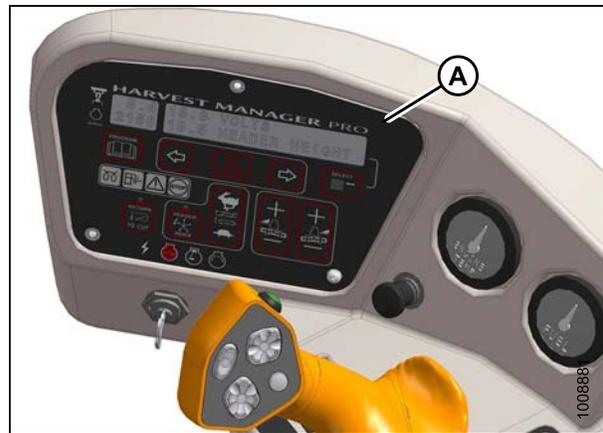
Figure 5.20: M155/M205 Cab Display Module (CDM)
