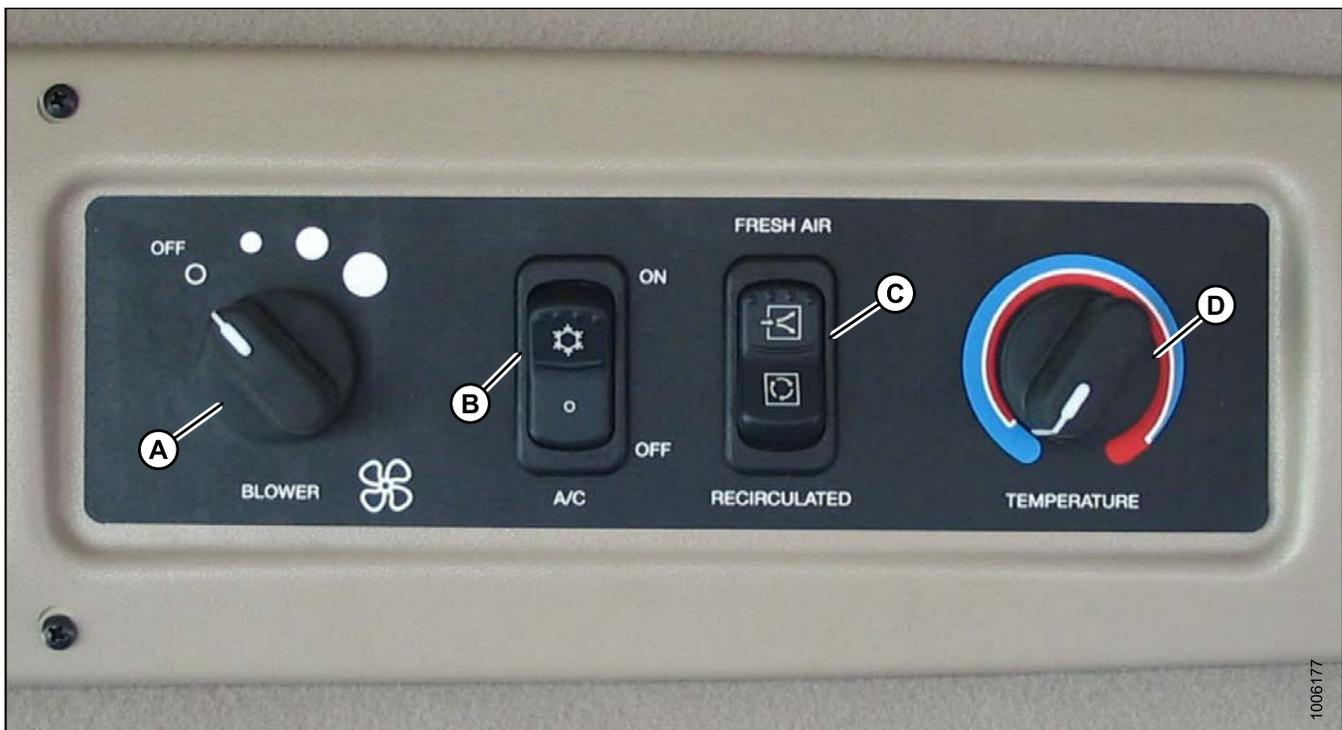
Figure 5.31: M155/M205 A/C and Heater Controls
