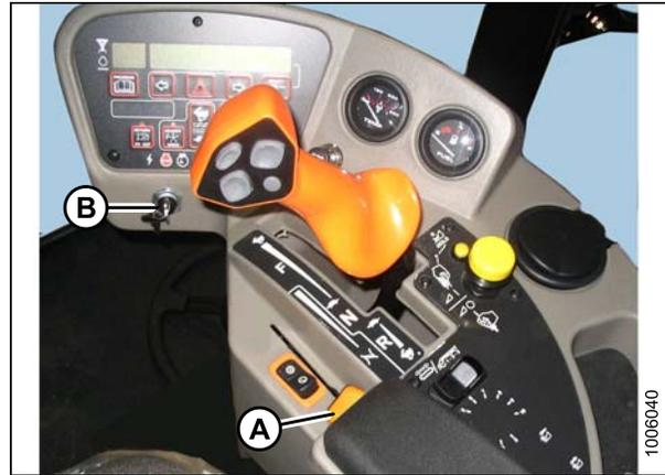
Figure 3.23: Operator Console
