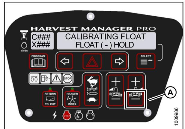
Figure 4.51: Negative Header Float
