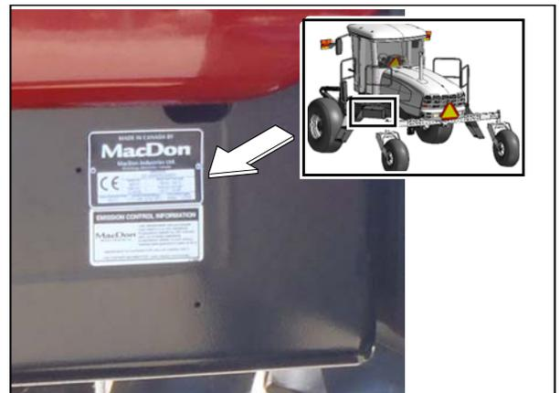
Figure 5.1: Serial Number Plate
