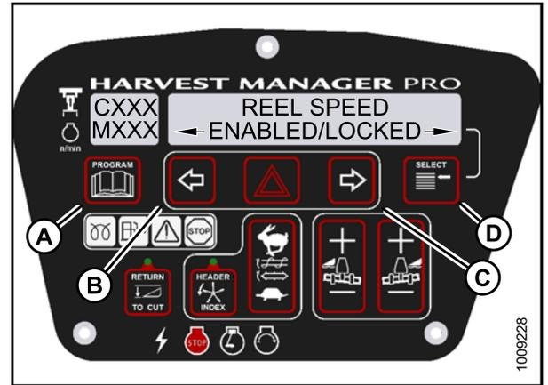
Figure 4.146: Reel Speed Control Lock
