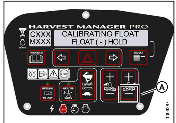
Figure 4.50: Negative Header Float
