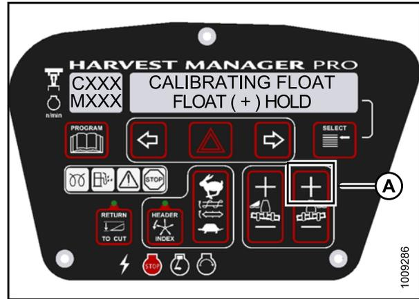
Figure 4.48: Positive Header Float
