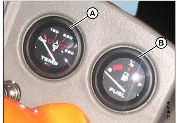
Figure 5.21: M155/M205 Temperature and Fuel Gauges
