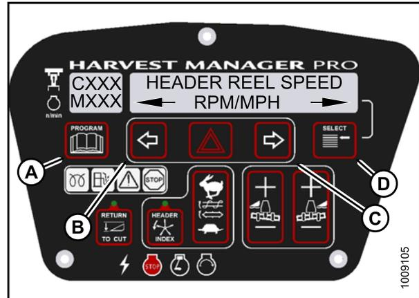
Figure 4.99: Reel Speed Display
