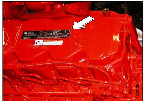
Figure 5.2: Engine Serial Number Plate
