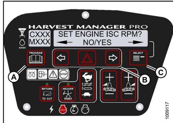
Figure 4.107: Engine ISC RPM
