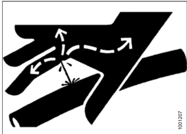
Figure 1.12: Hydraulic Pressure Hazard
