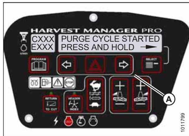
Figure 5.155: Hydraulic Purge Cycle
