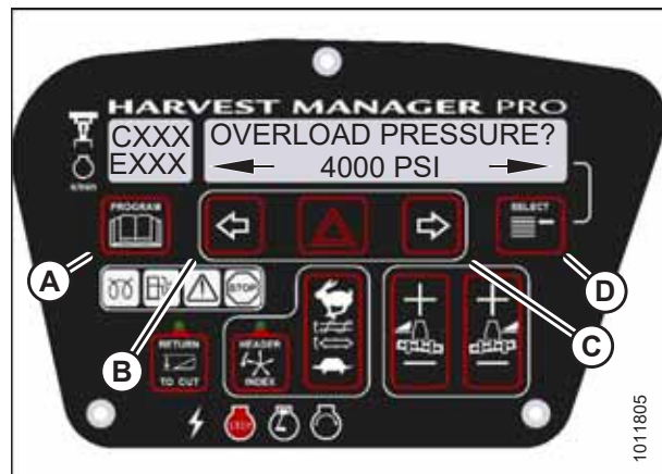
Figure 5.24: Hydraulic Overload Pressure
