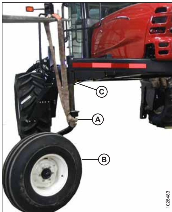
Figure 3.10: Caster Wheel Supported by Sling
