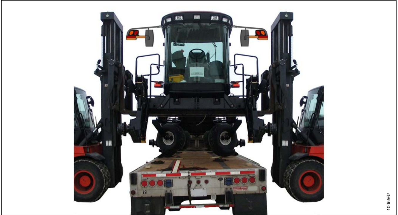
Figure 2.1: Two-Forklift Unloading Method
