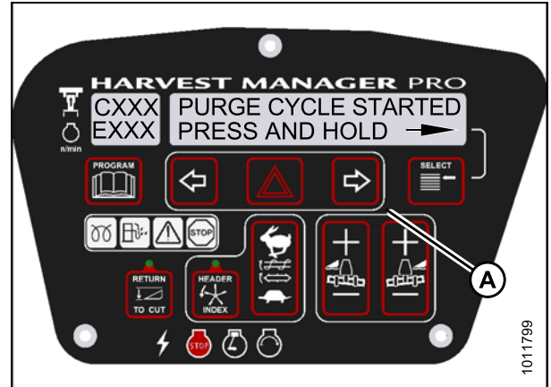
Figure 4.123: Hydraulic Purge Cycle
