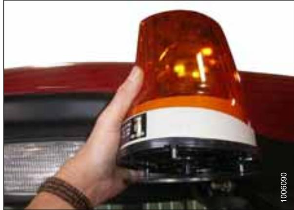
Figure 3.82: Beacon Light Orientation
