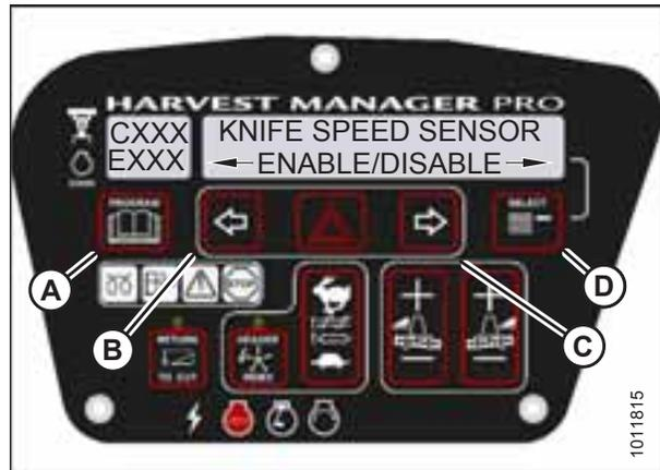
Figure 4.107: Header Sensors
