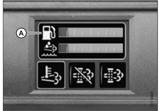
Figure 5.9: Fuel and DEF Gauges
