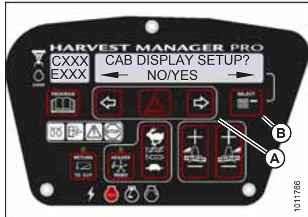
Figure 4.12: Cab Display Setup
