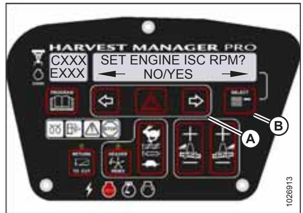
Figure 4.52: Engine ISC RPM
