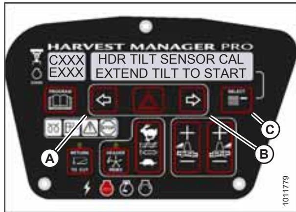
Figure 4.88: Header Tilt Calibration
