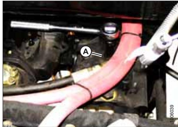
Figure 3.126: Traction Drive Pump Housing
