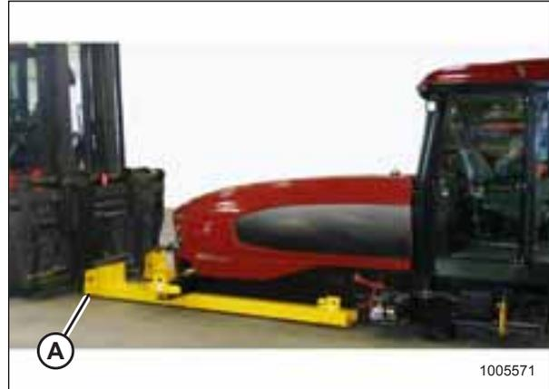
Figure 3.6: Forklift Method Lifting Points
