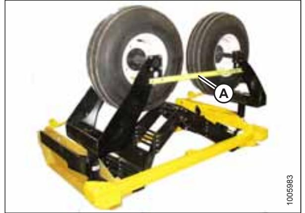
Figure 3.20: Caster Wheel Shipping Assembly
