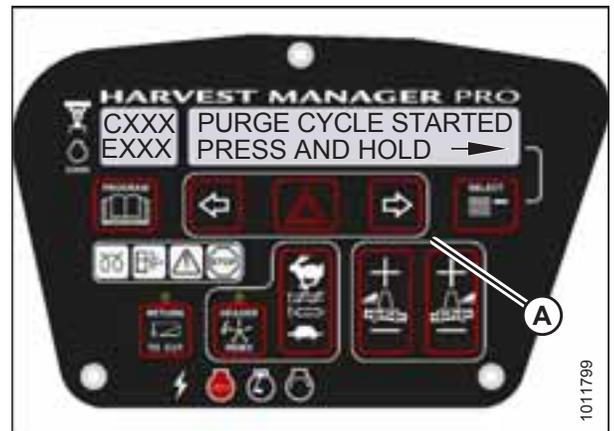
Figure 4.155: Hydraulic Purge Cycle
