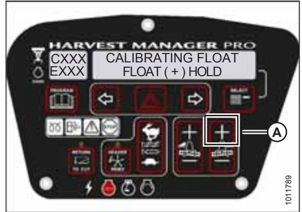
Figure 4.94: Positive Header Float Display
