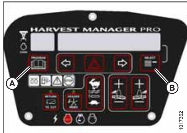
Figure 4.54: Cab Display Module (CDM)
