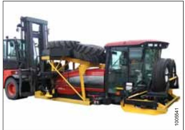
Figure 2.6: Forklift Method Lifting Points
