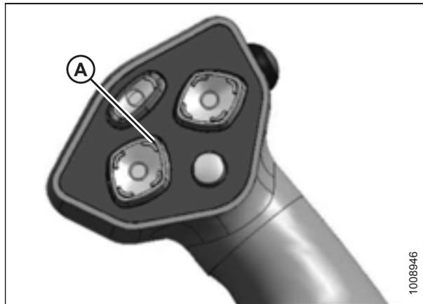
Figure 6.25: Ground Speed Lever
