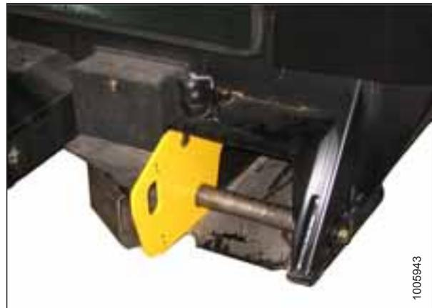
Figure 2.16: Lifting Plate
