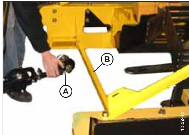
Figure 2.15: Wheel/Step Assembly Frame
