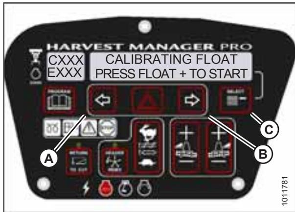
Figure 4.93: Header Float Display
