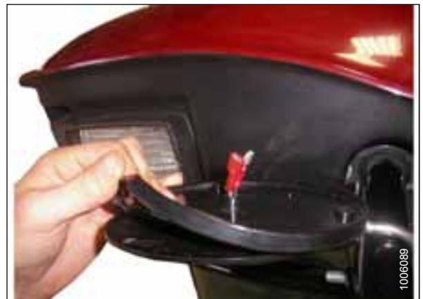
Figure 3.80: Rubber Beacon Base on Mounting Bracket
