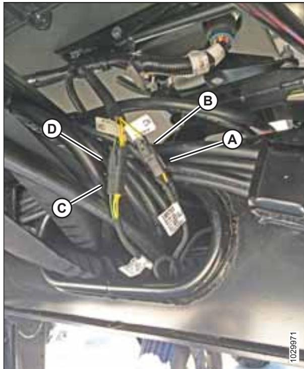
Figure 3.37: Wheel Leg Harness Connections
