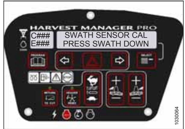
Figure 4.99: Swath Compressor Sensor Calibration
