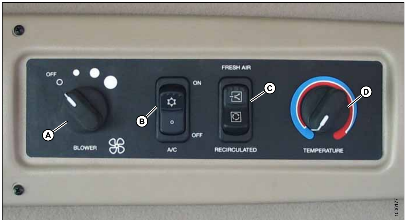
Figure 5.17: A/C and Heater Controls
