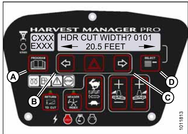
Figure 4.36: Header Cut Width
