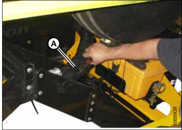
Figure 2.12: Hose Bundles on Frame
