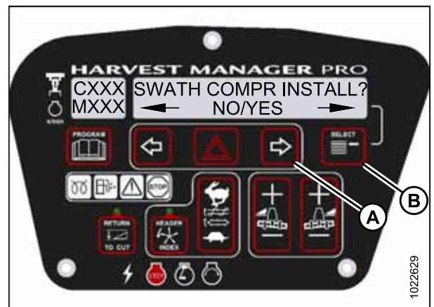
Figure 4.38: Swath Compressor Controls
