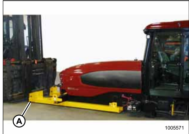
Figure 3.6: Forklift Method Lifting Points
