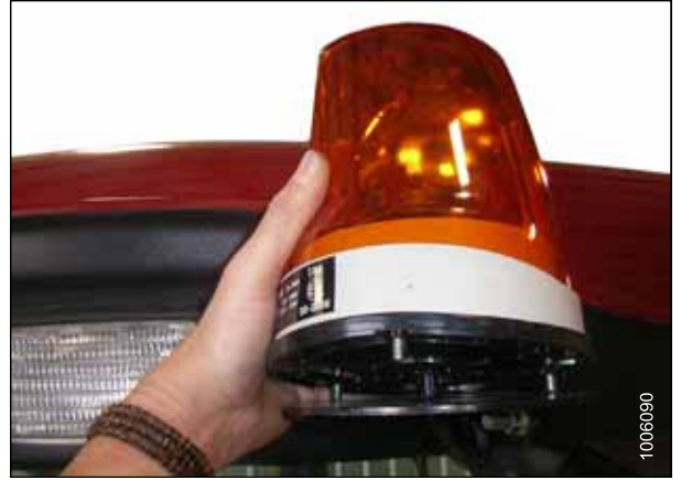
Figure 3.90: Beacon Light Orientation
