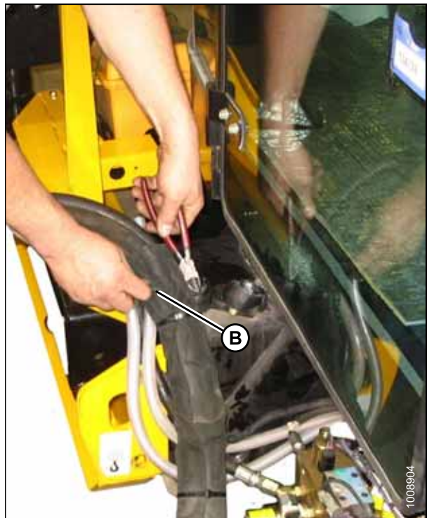
Figure 2.13: Hose Bundles on Frame
