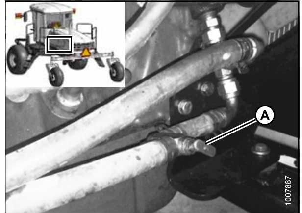
Figure 3.33: Heater Shut-Off Valve
