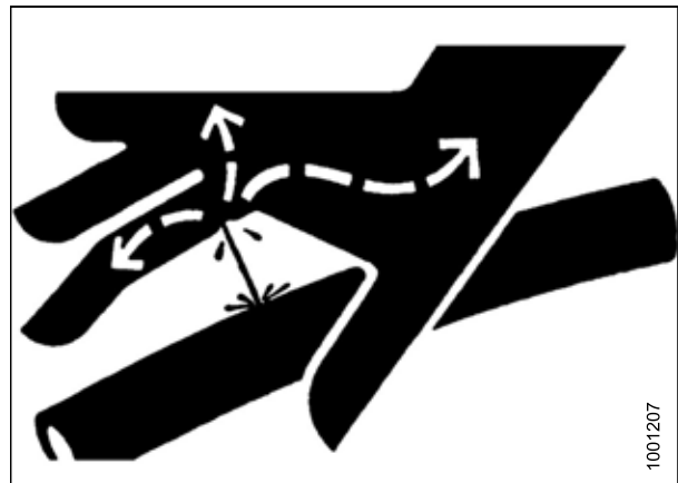
Figure 1.12: Hydraulic Pressure Hazard
