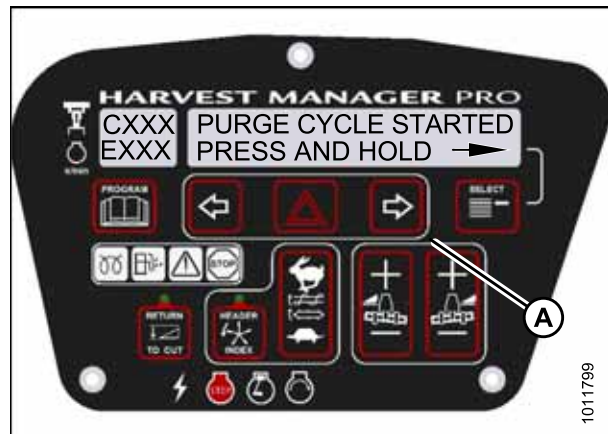
Figure 3.232: Hydraulic Purge Cycle
