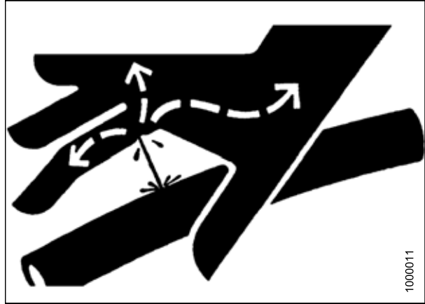
Figure 5.195: Hydraulic Pressure Hazard
