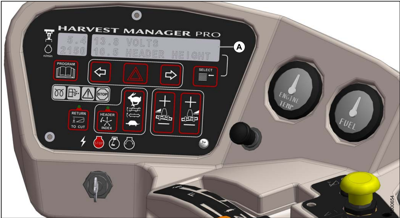
Figure 3.64: CDM Display Warnings and Alarms
