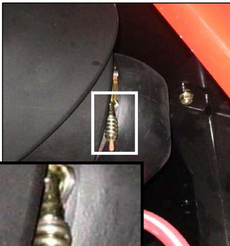
HOLD 0.018 in. (0.46 mm) GAUGE BETWEEN MIDDLE COILS AND TIGHTEN CLAMP UNTIL GAUGE IS SNUG.
