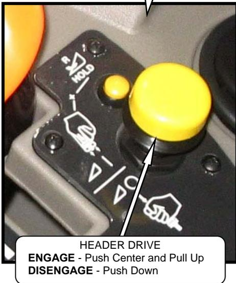
Engages and disengages header drive.
