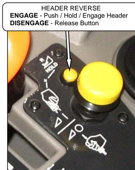
2. Push down and hold header drive reverse button, and pull up the header drive switch.
