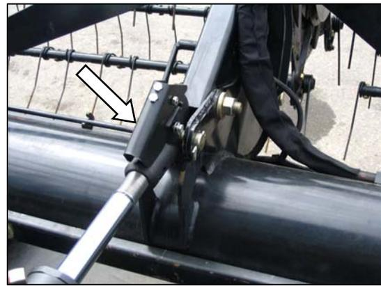
2. Lower the center-link onto the header with REEL DOWN switch until it locks into position (handle is down).
