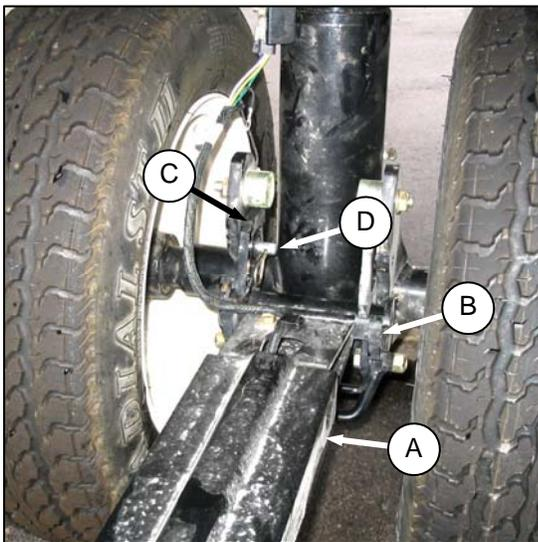
1. Position end (A) of the aft section onto front wheel hook (B).
