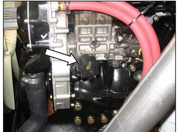
1. Turn cap counter clockwise, and remove filler cap.
