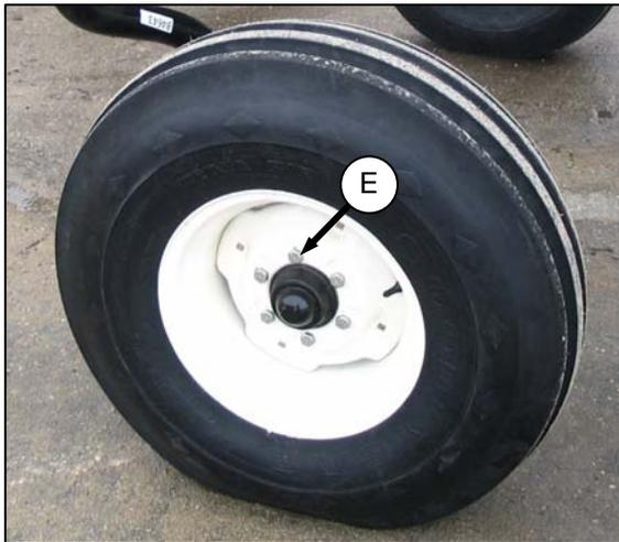
4. Undo the six wheel bolts (E), and remove wheel from hub.
