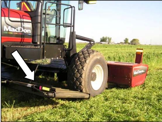
The double windrow attachment (DWA) allows the combining of two windrows of conditioned material close together to be picked up by a forage chopper. This unit may be mounted on the MacDon M150 and M200 Windrowers.
