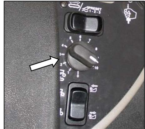
The drums are hydraulically driven, and the rotational speed can be varied from 0 to 1000 rpm from the windrower cab with the rotary knob on the Operator's console.
