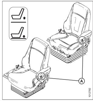
Figure 3.6: Operator's Seat Suspension and Height Controls
