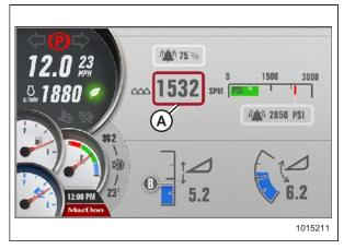
Figure 4.231: Setting Knife Speed
