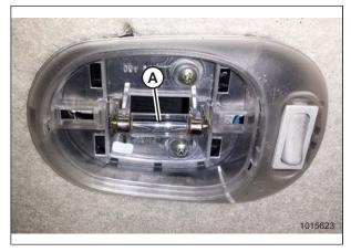
Figure 5.164: Cabin Dome Light with Cover Removed
