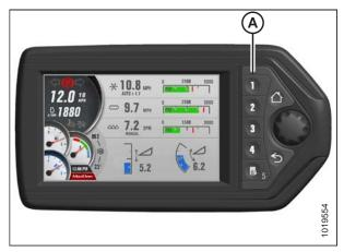
Figure 4.223: Header Run Screen 1
