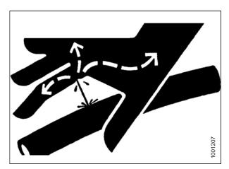
Figure 1.12: Hydraulic Pressure Hazard
