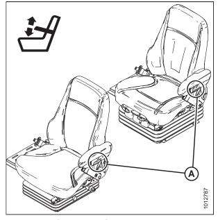
Figure 3.5: Operator's Seat Armrest Angle Controls
