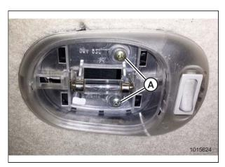
Figure 5.167: Cabin Dome Light with Cover Removed
