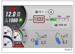
Figure 4.239: Adjusting Knife Speed Alarm
