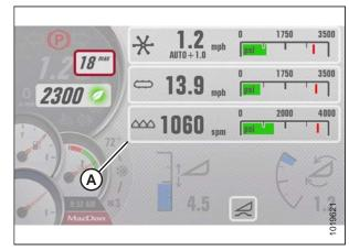
Figure 4.234: Draper Header QuickMenu
