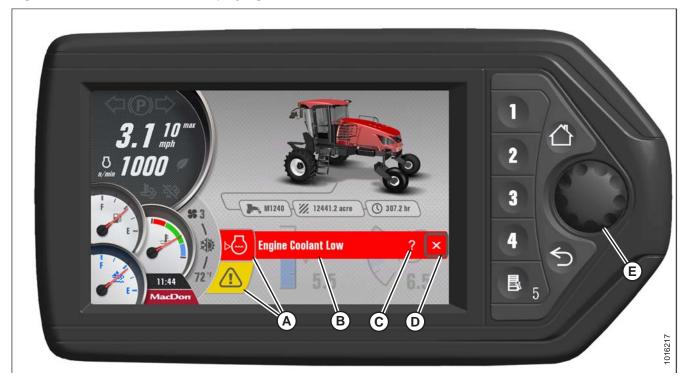
If multiple faults are detected, the number of faults will appear in the corner of the telltale icon (A).
