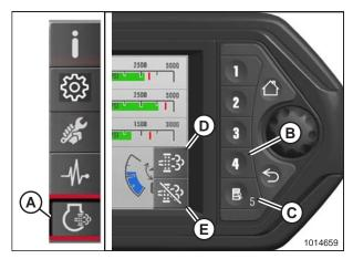
Figure 3.92: Engine Aftertreatment Icon and Soft Keys
