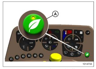
Figure 4.19: Eco Engine Control (EEC) Button
