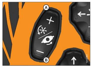
Figure 3.61: GSL Reel and Disc Speed Switch
