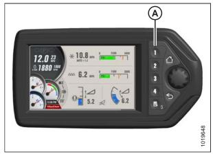
Figure 4.267: Header Run Screen 1
