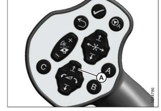
Figure 4.156: Ground Speed Lever
