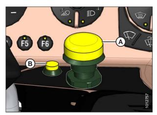
Figure 3.55: Header Drive Controls
