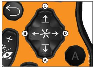
Figure 3.60: Ground Speed Lever
