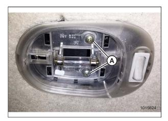
Figure 5.169: Cabin Dome Light with Cover Removed
