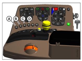
Figure 3.131: Operator's Console Shortcut Buttons
