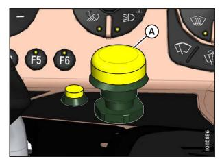
Figure 4.245: Header Engage Switch
