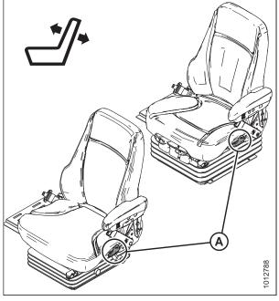
Figure 3.9: Operator's Seat Tilt Controls
