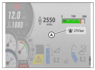
Figure 4.285: Disc Pressure Screen
