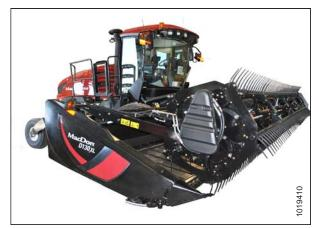
Figure 4.54: Windrower with Header
