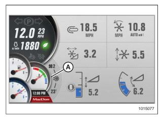
Figure 4.21: HPT Display – Engine Temperature Gauge
