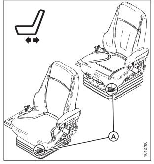
Figure 3.7: Operator's Seat Fore-Aft Position Controls
