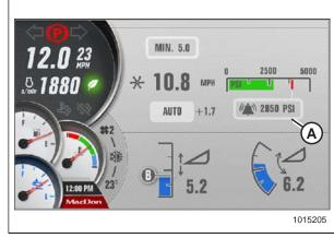
Figure 4.262: Setting Reel Alarm Pressure
