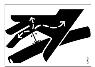
Figure 5.37: Hydraulic Pressure Hazard
