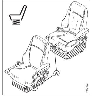
Figure 3.11: Operator's Seat Vertical Dampener Controls
