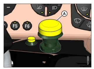
Figure 4.277: Header Engage Switch
