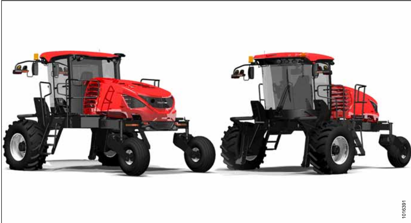
M1170 Windrower, featuring Dual Direction® and Crossflex™ rear suspension
