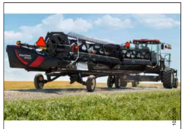
Figure 4.49: Towing a Header
