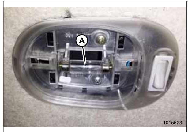
Figure 5.181: Cabin Dome Light with Cover Removed
