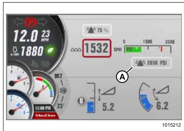
Figure 4.239: Adjusting Knife Alarm Pressure
