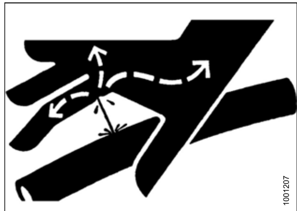
Figure 1.12: Hydraulic Pressure Hazard
