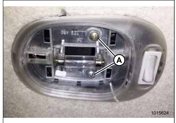
Figure 5.186: Cabin Dome Light with Cover Removed
