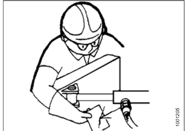
Figur 1.11: Test for hydrauliklækager
