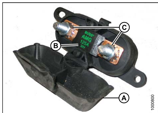
Figure 5.171: 125A Main Fuse
