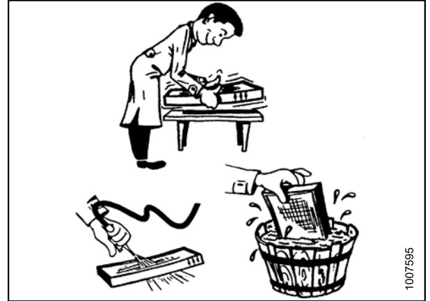
Figure 5.46: Cleaning the Fresh Air Filter
