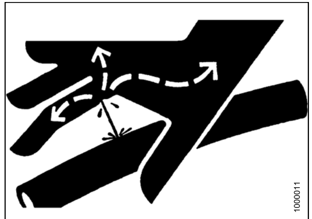
Figure 5.173: Hydraulic Pressure Hazard
