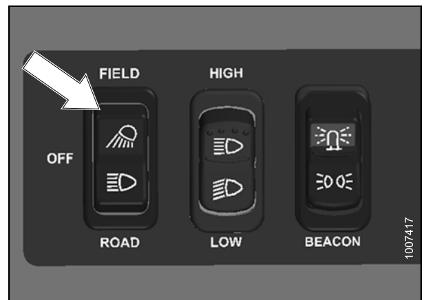
Figure 3.8: Field Light Switch
