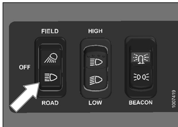
Figure 3.11: Road Lighting Switch
