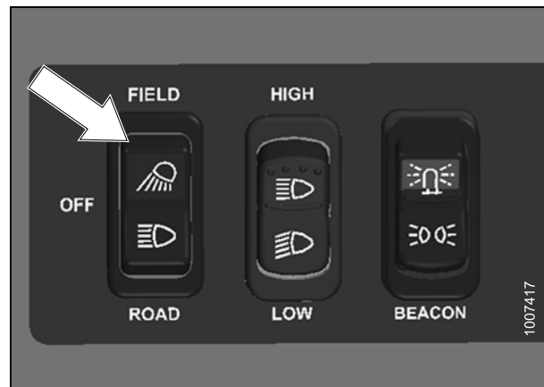
Figure 3.16: Field Light Switch
