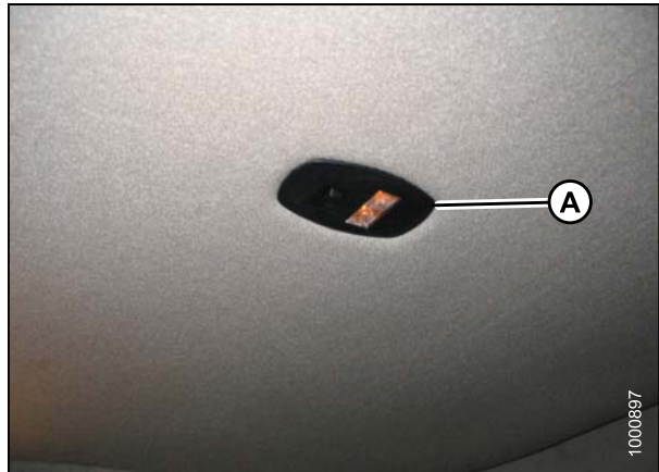
Figure 5.164: Ambient Light Fixture
