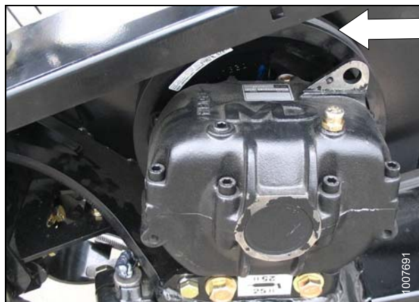
Figure 4.184: Knife Drive Box on Header
