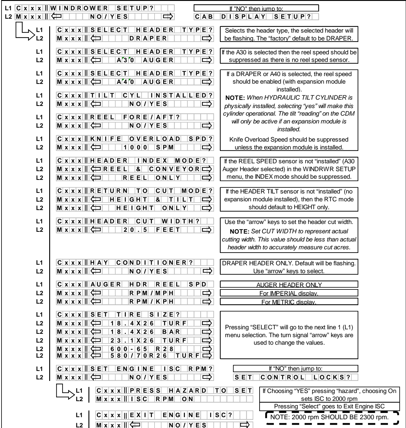
Programming Menu Flow Chart for Software version C107 and M102 (or higher)
