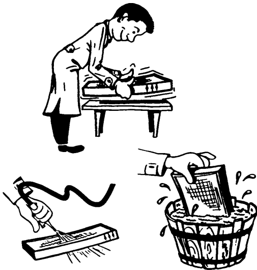
CLEANING AIR FILTER
