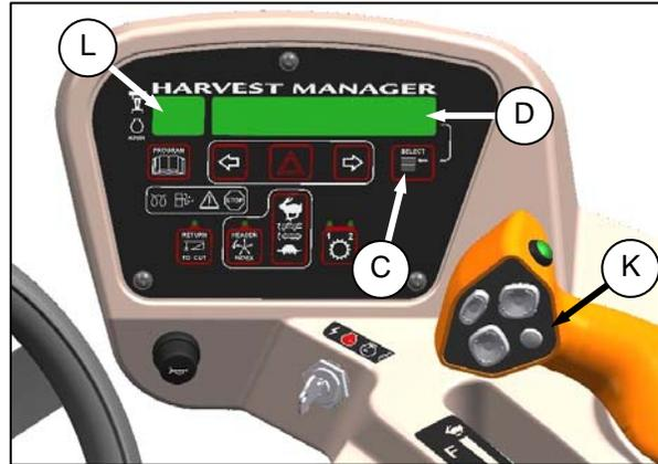
Check CDM display (D) is working by pushing SELECT (C) on CDM or SELECT button (K) on GSL.
