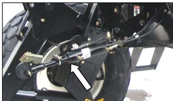
The hydraulic center link is supplied in a separate kit that is included with the shipment. Refer to installation instructions in the kit.
