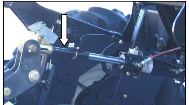
5. Push down on rod end of link cylinder until hook engages pin on header and is locked.
