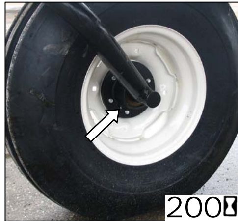
FORMED CASTER WHEEL BEARING 1 PLACE (BOTH WHEELS)
