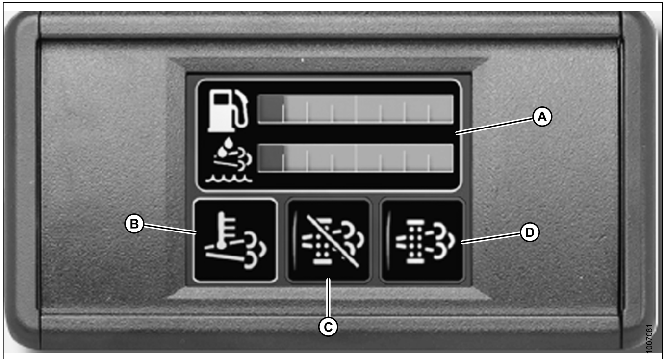
Figure 5.1: Fuel and Diesel Exhaust Fluid (DEF) Display Module
