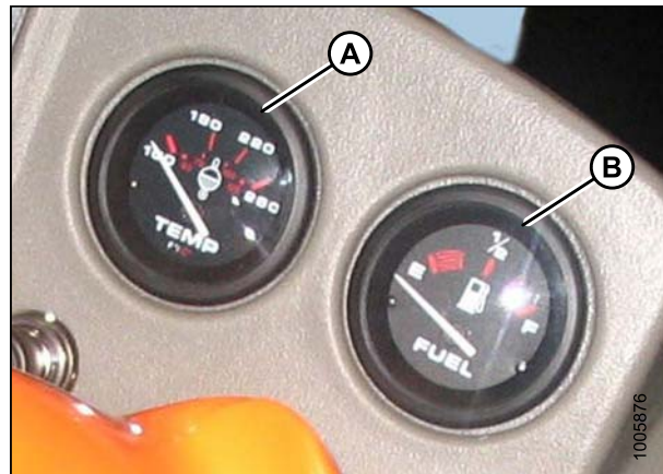
Figure 5.29: M155/M205 Temperature and Fuel Gauges
