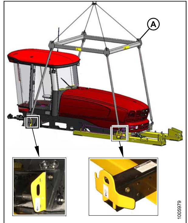
Figure 3.4: Shipping Frame Lifting Points
