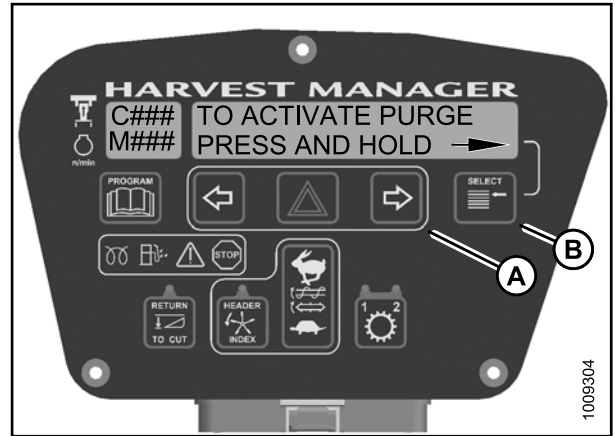
Figure 4.335: M105 Hydraulic Purge
