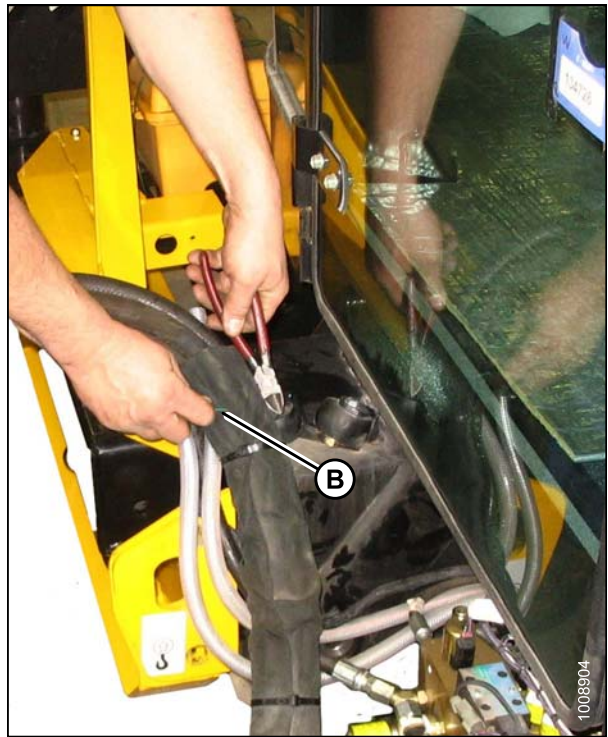
Figure 2.13: Hose Bundles on Frame
