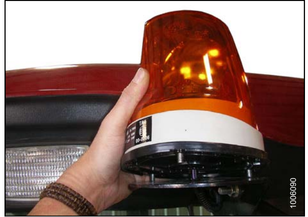
Figure 3.149: Beacon Light Orientation
