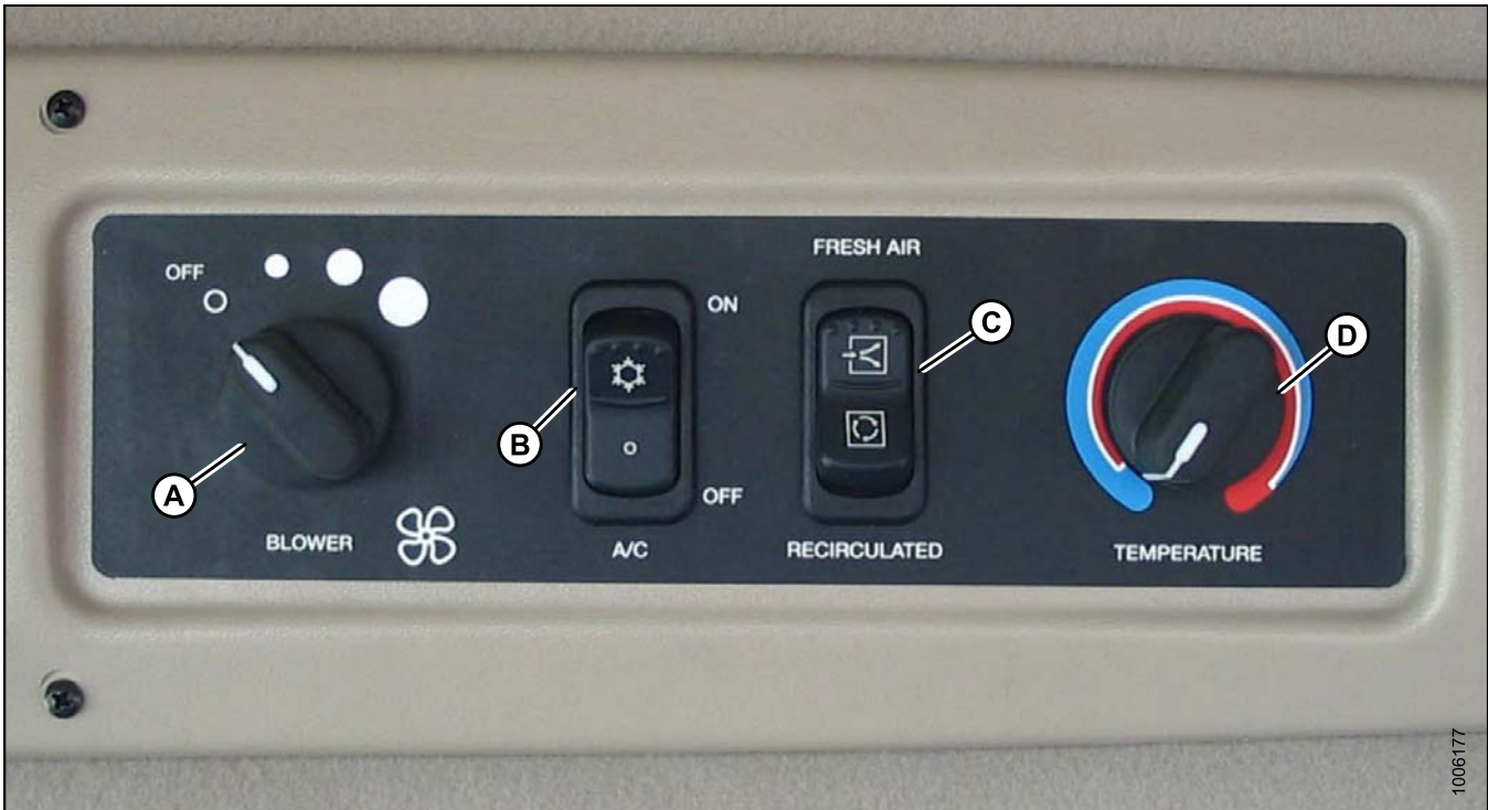
Figure 5.46: M155/M205 A/C and Heater Controls
