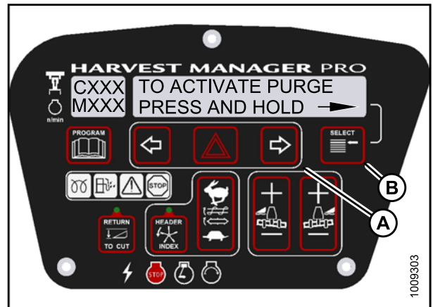
Figure 4.336: M155 Hydraulic Purge
