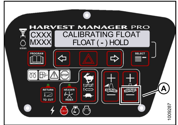
Figure 4.70: M155 Negative Header Float
