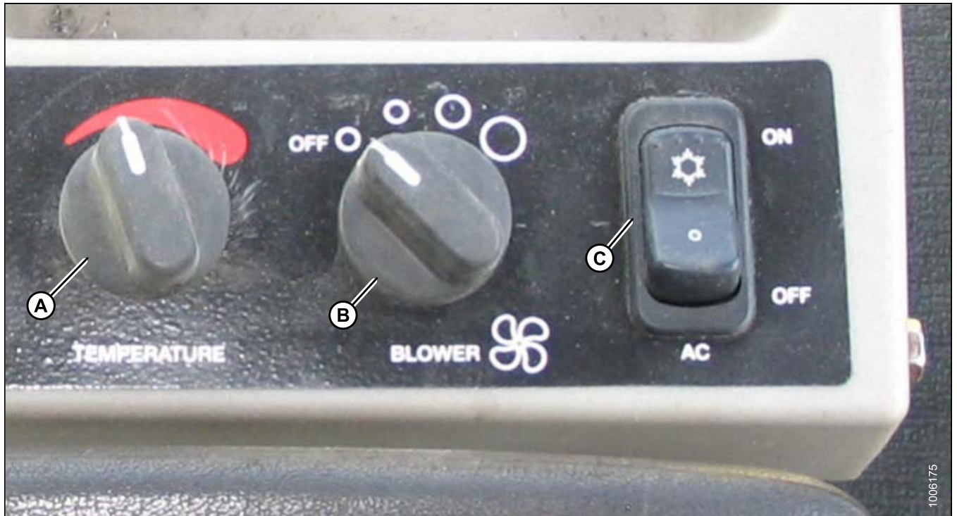
Figure 5.47: M105 A/C and Heater Controls
