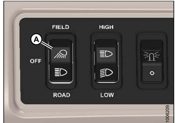
Figure 7.33: Exterior Light Switches
