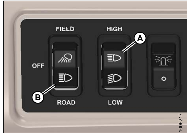
Figure 7.47: Exterior Light Switches
