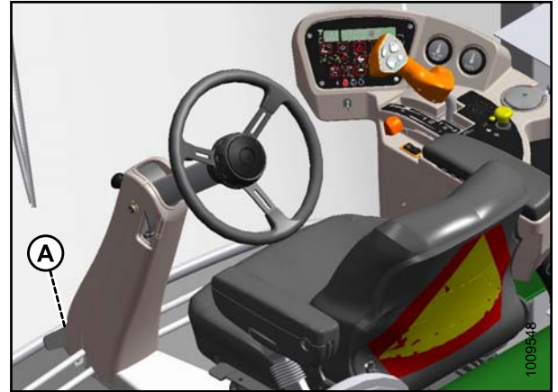
Figure 6.129: M155/M205 Operator Console
