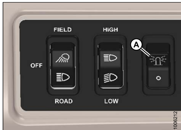
Figure 7.42: Exterior Light Switches
