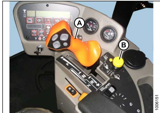
Figure 7.31: M155/M205 Operator Console
