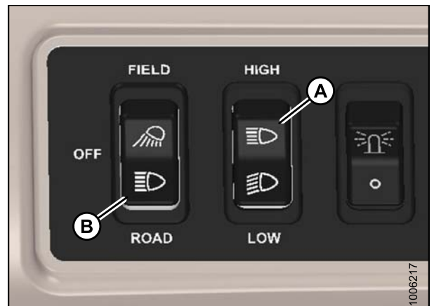
Figure 7.39: Exterior Light Switches
