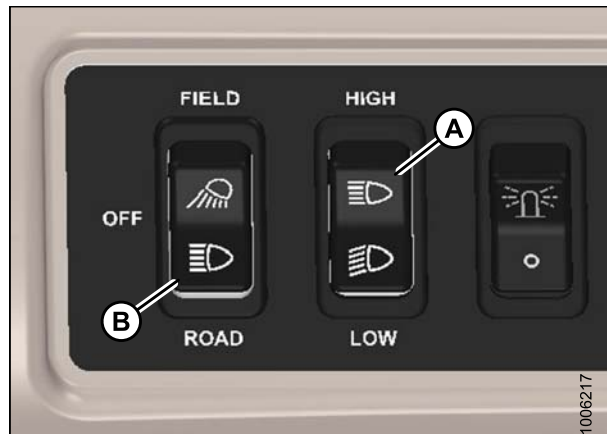
Figure 7.36: Exterior Light Switches
