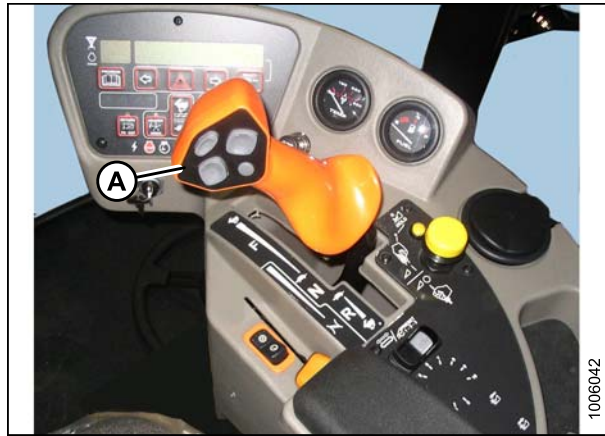
Figure 6.134: M155/M205 Operator Console
