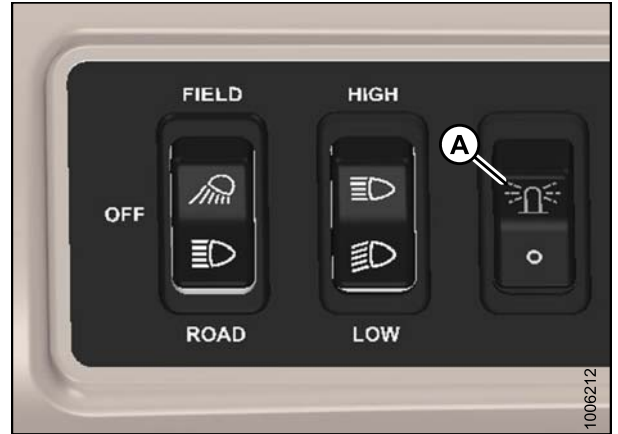
Figure 7.50: Exterior Light Switches
