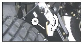
k. Disengage lift cylinder stops by turning lever (M) downward to release and lower stop until lever locks into vertical position. Repeat for opposite lift cylinder stop.
