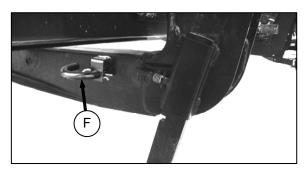
b. Remove hairpin on pins (F), and remove pins from header legs.
