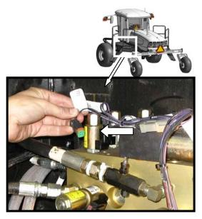
h. Disconnect brake engage solenoid connector (P-V3) at valve block on LH side of windrower.
