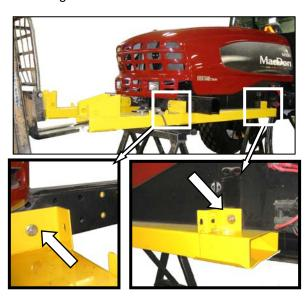
Support shipping frame channel, and remove bolts attaching shipping frame to walking beam and mainframe side rail. Remove shipping frame.
