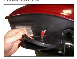
Feed connectors from harness through center hole in rubber base, and place base on beacon bracket - making sure mounting holes in rubber base line-up with holes in bracket.
