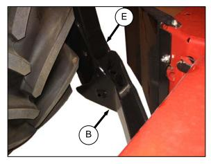
d. Slowly drive windrower forward so that feet (E) on windrower enter boots (B) on the header.
