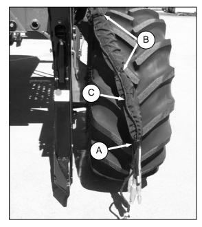
m. Undo strap (A), cut plastic cable ties (B), and move harness (C) away from hose bundle.
