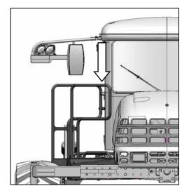
Slowly close platform, and check that vertical rail tubes are parallel with cab posts when viewing from the rear. Laterally adjust king pin mounting as required.
