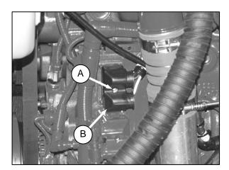
c. Remove socket head screw (A) with a 4 mm Allen wrench, and remove ECM connector (B) from engine. This prevents engine from starting during cranking.
