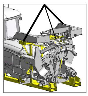
b. To prevent paint damage, attach two slings and a chain to platform at locations shown, and to a lifting device with a minimum lifting capacity of 5,000 lb (2268 kg), and a lift height of 13 feet (4 m).
