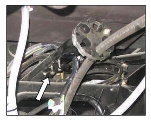
Locate hose clip under the cab, and remove clip.
