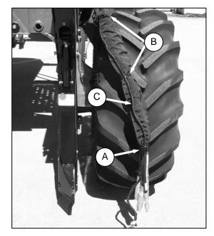
I. Undo strap (A), cut plastic cable ties (B), and move harness (C) away from hose bundle.
