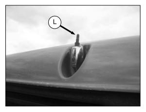
o. Remove protective cover (L) from antenna mount on cab roof and thread antenna onto base until hand tight.
