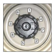
f. Install wheel nuts, and tighten to 220 ft-lbf (300 N·m) using the tightening sequence as shown above.
