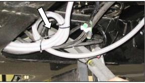
d. Feed hydraulic hose bundle into frame, and through hole at center of frame.
