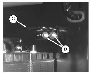
c. Remove one of the two bolts (D) and nuts, and loosen the other.
