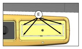
d. Remove the cut-out by cutting the tabs (E) in the panel. Remove sharp edges on panel.
