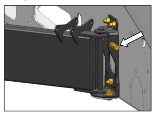
k. Adjust platform horizontally with the 1/2 in. x 2.25 bolt as required.
