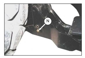
h. Install pin (N) through each boot and foot, and secure with hairpin.
