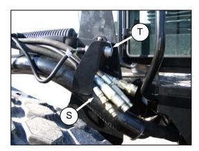
r. Connect header drive hydraulics (S) and electrical harness (T) to header. Refer to Auger Header Operator's Manual.
