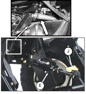
Adjust position of the center-link cylinder (E) with the REEL UP and REEL DOWN switches, and HEADER TILT switches on the GSL to position the hook above the header attachment pin.
