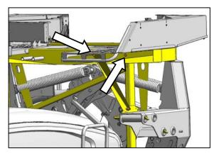
c. Remove two 5/8 in. x 5.0 bolts at top of vertical supports, and two 5/8 in. x 1.25 bolts attaching angle braces to platforms.
