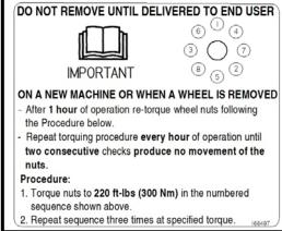
b. Remove decal (166497) from windshield **ONLY** after machine is delivered to end user.
