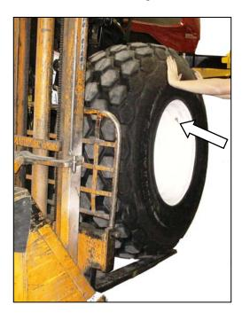
Position wheel against hub so that that air valves are on the outside, and tire tread points forward.
