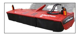
The M205 is factory-equipped with hydraulics and connections to run the R-Series Rotary Disc headers.
