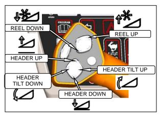
f. If engine is not running, start engine. Press HEADER UP switch to raise header to maximum height.
