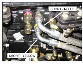
Remove caps, and attach hoses with short elbows to respective side of pump (either yellow or no tie). Tighten fittings.
