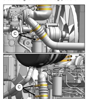
e. Check constant torque clamps (C) on charge air cooling duct connections at turbocharger outlet and engine air intake. Clamps (C) should be tightened to achieve gap as shown opposite.
