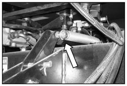
1. If the optional center-link self-alignment kit is installed, activate the REEL UP switch on the GSL to raise the center-link (G).
