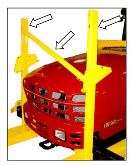
a. Remove cross brace, and the two upright supports from frame.
