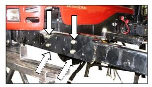
j. Install six 3/4 in. bolts and hardened washers into walking beam and caster beam. Use longer bolts through anti-shimmy bracket.
