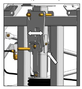
Ensure that the three (one at rear, two at front) lift locks are activated on lift mechanism.
