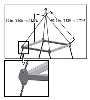
a. Attach chains or cable to the four lift points on the lifting frame (MacDon Part # 163871) and connect loop ends to crane hook. Use cable or chain with a minimum lifting capacity of 7100 lb (3221 kg).
