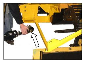
h. Lift center-link so that it clears wheel/step assembly frame.
