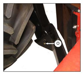
i. Install pin (O) through each boot and foot, and secure with hairpin.
