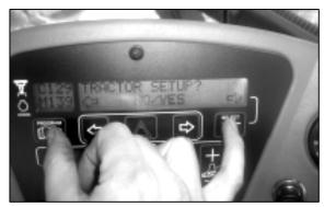
Simultaneously press the PROGRAM and SELECT buttons to bring up the TRACTOR SETUP screen.
