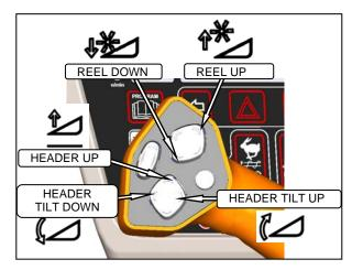
d. Adjust the position of the center-link cylinder with the REEL UP and REEL DOWN switches, and HEADER TILT switches on the GSL to position the hook above the header attachment pin.
