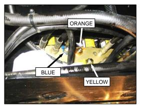
13. Remove the caps from three fittings (blue, orange, and yellow ties) on the valve block from inboard side of frame.
