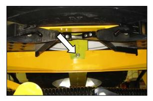
b. Remove one bolt at rear of hood directly under center of drive wheel.
