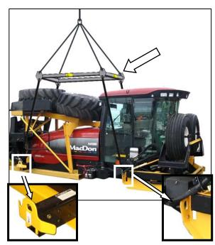
b. Attach lifting frame assembly (MacDon Part #163871) to the four designated lift points on windrower shipping frame.
