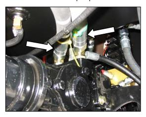
1. Remove caps, and attach hoses (green and yellow ties) to matching fittings on top of pump. Tighten fittings.
