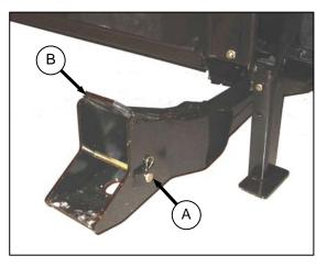
a. Remove hairpin from pin (A), and remove pin from left and right header boots (B) on header.
