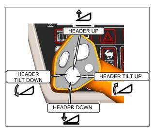
Start the engine, and activate HEADER DOWN button on the GSL to fully retract header lift cylinders.
