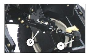
g. If necessary, adjust position of the hydraulic center-link (G) so that the hook (H) is above the attachment pin on the header by one of the following methods:
