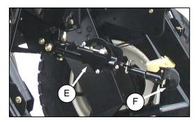
c. If necessary, adjust position of the hydraulic center-link (E) so that the hook (F) is above the attachment pin on the header by one of the two following methods (shown in next column):
