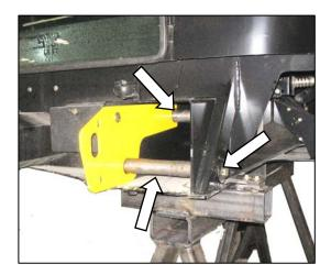
a. Remove front leg bolts and pins, and set aside for re-installation. Remove carriage bolt, and remove lifting plate.
