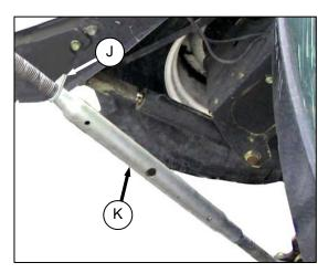
Loosen nut (J), and rotate barrel (K), to adjust length so that other end lines-up with header bracket.
