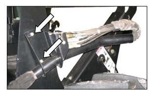
t. Attach reel hose support tube to the RH reel leg with two 3/8 in. x 1.0 carriage bolts and nuts.
