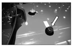
Remove hydraulic oil reservoir filler cap/dipstick.
