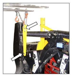
b. Attach chain to lifting bar on leg assembly, and hook up to lifting device with a minimum lifting capacity of 5,000 lb (2,268 kg).
