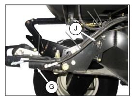
2. Without the self-alignment kit, re-locate the pin (J) at the frame linkage as required to raise the center-link (G).
