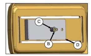
Remove screw and nuts (B) and (C) to remove support (D) from panel. Retain metric nut (C) and lock washer.
