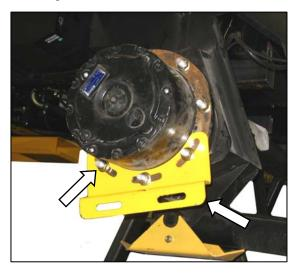
b. Remove shipping supports on drive wheel hubs, and remove wheel lug nuts.
