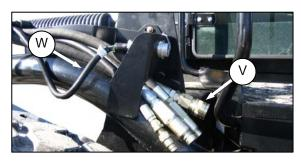
s. Connect header drive hoses (V) and electrical harness (W) to header. Refer to the Draper Header Operator's Manual.
