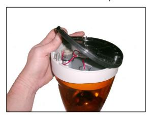
b. Remove hardware and rubber base from one of the beacons as shown.
