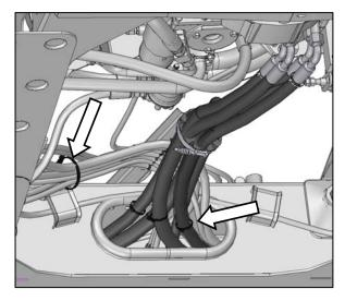
v. Secure hoses with cable ties as required.
