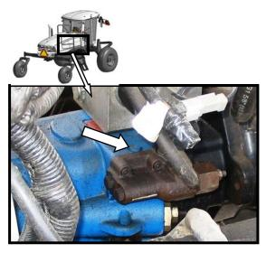
c. Locate plug on TOP of HEADER drive pump housing from above, and loosen plug to bleed pump housing. Re-tighten plug once oil starts to run out.
