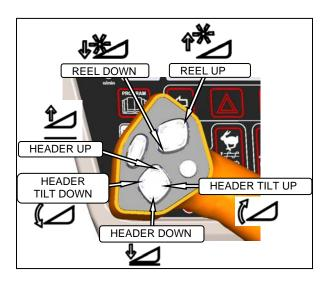
k. If engine is not running, start engine, and press HEADER UP switch to raise header to maximum height.
