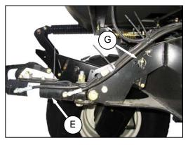
2. Without the self-alignment kit, re-locate the pin (G) at the frame linkage as required to raise the center-link (E).
