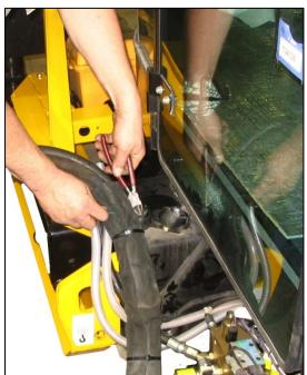
f. Remove plastic cable tie and shipping wire securing hose bundles to frame.
