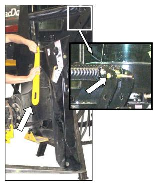
h. Slightly lift the header lift arms with lifting device, and remove lifting bars from legs. Relocate spring locking pins to front of lift arms.
