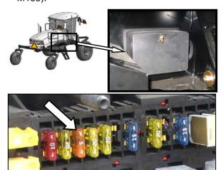
k. Open circuit breaker/fuse box, and remove ECM ignition fuse (5A).
