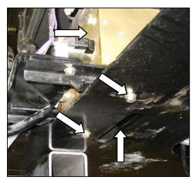
14. Loosen bolts, and move valve block to improve access through hole in frame for wrenches when tightening fittings.
