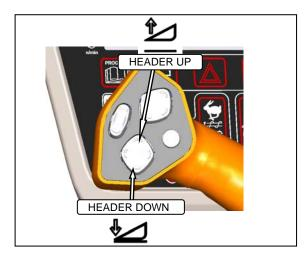
g. Start engine (if not running), and press HEADER UP switch to raise header to maximum height.
