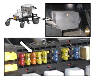
i. Open circuit breaker/fuse box, and remove ECM ignition fuse (5A).
