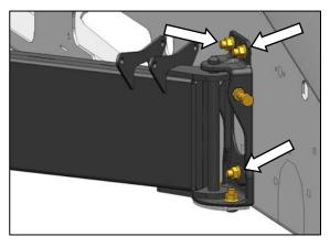
e. Attach main beam of platform to side frame with three 1/2 in. x 1.25 long carriage bolts. Bolt heads face inboard. Tighten just enough for adjustment.
