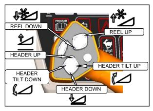
f. Start engine, and activate HEADER DOWN button on the GSL to fully retract header lift cylinders.
