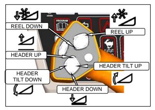
p. Start engine, and activate HEADER DOWN switch on GSL to lower header fully.
