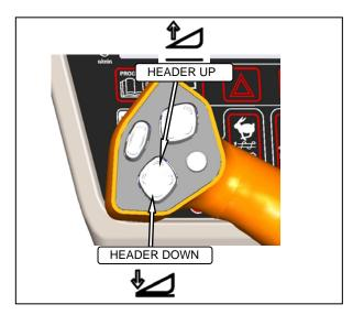
Start engine, and activate HEADER DOWN switch on GSL to lower header fully. Stop engine, and remove key.
