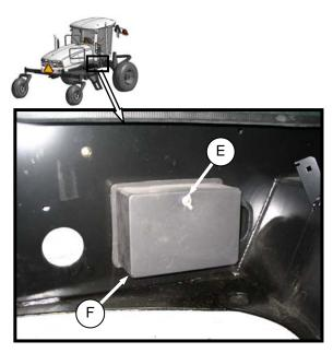
a. Remove wing nut (E) from fuse box cover (F) and remove cover.
