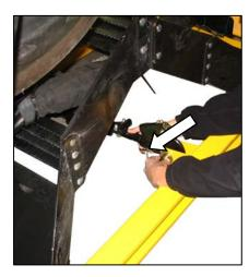
d. Remove the 1 inch (25.4 mm) pin at the center-link.
