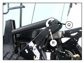
m. Remove pin (Q) from storage position in linkage, and insert in hole (R) to engage float springs. Secure with lynch pin.
