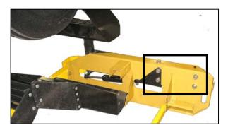
g. Remove five remaining bolts securing caster to shipping frame. Retain bolts for attaching caster to walking beam.
