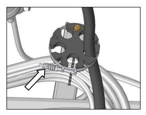
m. Remove clamp from round plastic hose block. Case drain hose is pre-installed in block.
