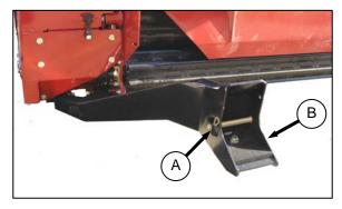
b. Remove hairpin from pin (A), and remove pin from on left and right header boots (B) on header.
