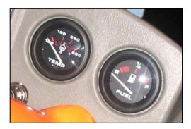
a. Check engine temperature gauge and fuel gauge are working (M205, M155 ONLY).
