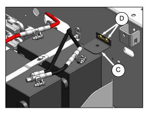
Rotate angle (C) 180 degrees, align holes, and reinstall the bolt (D) and nut. Leave bolts loose.
