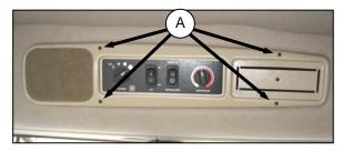
Remove radio panel by removing four screws (A).
