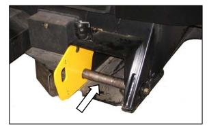
i. Re-install leg bolts, washers, and nuts to secure the lifting plate onto the mainframe.
