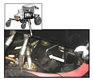
d. Locate plug on TOP of HEADER drive pump housing from above, and loosen plug to bleed pump housing. Re-tighten plug once oil starts to run out.
