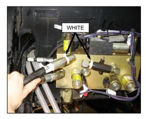
12. Remove caps on hose, and valve block fitting (white tie), and make connection. Tighten fitting.
