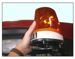
e. Fit beacon onto base making sure beacon is oriented as shown, with the point on lens facing forward (Cab-Forward).
