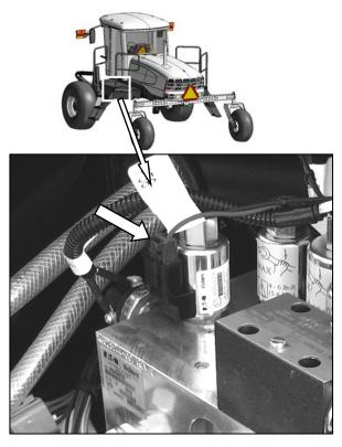
b. Disconnect brake engage solenoid (plug P44) at valve block on LH side of windrower.
