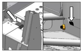
j. Check that rubber bumper is contacting the frame, and that front of platform is contacting the guide.
