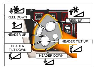
Start engine, and activate HEADER DOWN button on the GSL to fully retract header lift cylinders.
