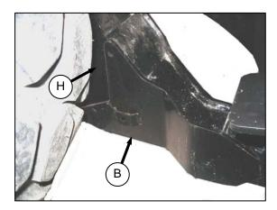
d. Slowly drive windrower forward so that feet (H) on windrower enter boots (B) on the header. Continue to drive slowly forward until feet engage the boots, and header nudges forward.
