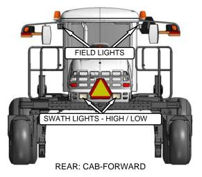
c. Switch ROAD lights ON, and check that all lights are functioning as shown below:
