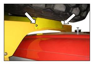
Remove the two bolts at front cross member over the hood.
