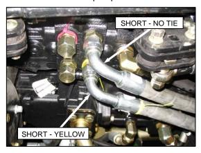
1. Remove caps, and attach hoses with short elbows to respective side of pump (either yellow or no tie). Tighten fittings.
