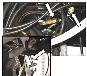
f. Retrieve the two motor case drain hoses (MD #111312) at front frame, and the 7/8 in. tee fitting on the hose, from the pump.
