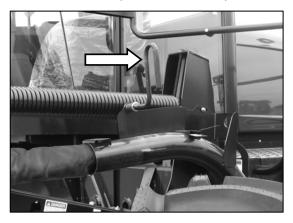
q. Disengage hook, and rotate to up position. Position hose bundle over hose support, and locate under hook.
