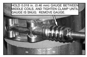
c. Constant torque spring type clamps (A) and (C) should be tightened to achieve gap as shown.
