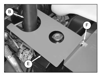
e. Position stack (B) in slot in exhaust shroud (E), and connect stack (B) to muffler (D).
