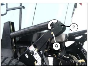
j. Remove pin (P) from storage position in linkage, and insert in hole (Q) to engage float springs. Secure with hairpin.
