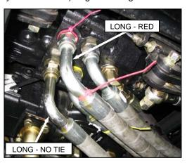
2. Remove caps, and attach hoses with long elbows to respective side of pump (either red or no tie). Tighten fittings.
