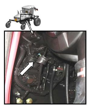
h. Disconnect electrical connection at fuel pump on right side of engine.
