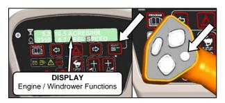
b. Check CDM display is working by pushing SELECT on CDM, or SELECT button on GSL.
