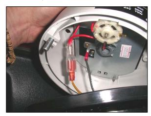
d. Connect orange wire from harness to the red wire in beacon. Black harness wire connects to ground terminal in beacon.
