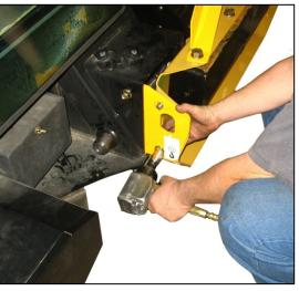
e. Remove the four (two per side) carriage bolts at the rear of the wheel/step assembly.
