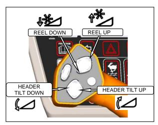
f. Adjust the position of the center-link cylinder with the REEL UP and REEL DOWN switches, and HEADER TILT switches on the GSL to position the hook above the header attachment pin.
