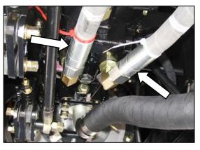
Remove caps, and attach hoses (red and white ties) to matching fittings on bottom of pump. Tighten fittings.
