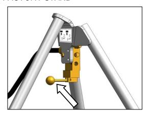
a. Move valve handle up to raise windrower slightly, and take load off lift locks.
