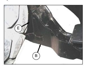
c. Slowly drive windrower forward so that feet (E) on windrower enter boots (B) on the header. Continue to drive slowly forward until feet engage the boots, and header nudges forward.
