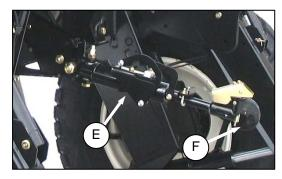
c. If necessary, adjust position of the hydraulic center-link (E) so that the hook (F) is above the attachment pin on the header by one of the following 2 methods (shown in next column):
