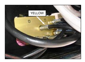
Remove the cap from fitting with yellow tie on the valve block from inboard side of frame.
