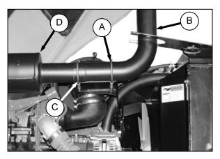
f. Tighten both clamps (A) and (C) but just enough so stack can be moved.
