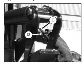
o. Attach harness (C) to hose support with hose clip (D).
