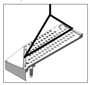
c. Attach a sling to platform, and other end to lifting device.
