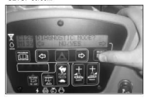
d. Push the SELECT button several times until the DIAGNOSTIC MODE screen is displayed.
