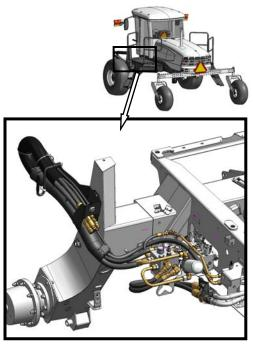
AUGER HEADER HYDRAULICS
