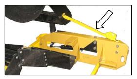
e. Remove the two braces from caster wheels and frame. Retain bolts for attaching caster to walking beam.
