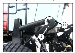
Remove pin (H) from storage position in linkage, and insert in hole (J) to engage float springs. Secure with lynch pin.
