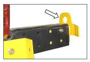
a. Remove the two guide plates from ends of walking beam.
