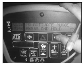
j. Press and hold the RIGHT ARROW button to activate and run the purge cycle until the purge is complete (approximately 1 minute). Release the ARROW button at any time to stop the cycle.
