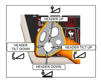
Start the engine, and activate HEADER DOWN button on the GSL to fully retract header lift cylinders.
