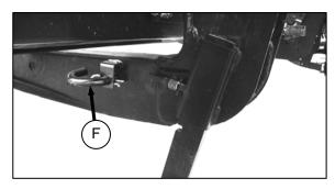
e. Remove hairpin on pins (F), and remove pins from header legs.
