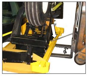
g. Attach a chain to wheel/step assembly, and pull away from shipping assembly with lifting device.
