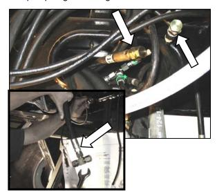
c. Retrieve the two motor case drain hoses (MD #111312) at front frame, and the 7/8 in. tee fitting on the hose from the pump.
