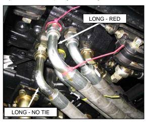
2. Remove caps, and attach hoses with long elbows to respective side of pump (either red or no tie). Tighten fittings.
