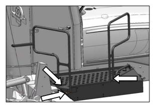
h. Attach railings to platform with 1/2 inch x 0.75 locking bolts provided. Tighten bolts to 75 ft·lbf. (102 N·m).
