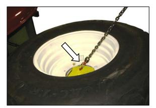
Attach a lifting device to lift hooks located in the center of each drive wheel.
