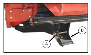
a. Remove hairpin from pin (A), and remove pin from on left and right header boots (B) on header.
