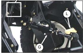
Adjust position of the center-link cylinder (G) with the REEL UP and REEL DOWN switches, and HEADER TILT switches on the GSL to position the hook above the header attachment pin.
