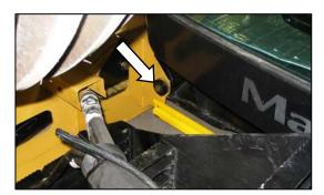
c. Remove the two 3/4 in. x 16.5 long bolts (one per side) at front frame beam. Retain for re-installation.
