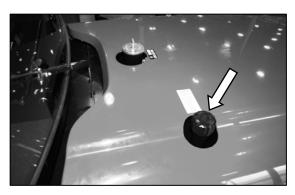
Check hydraulic oil level in reservoir. Add SAE15W-40 oil if necessary.
