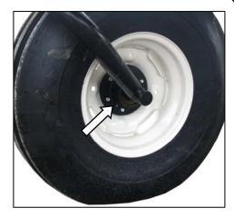
FORMED CASTER WHEEL BEARING 1 PLACE (BOTH WHEELS)
