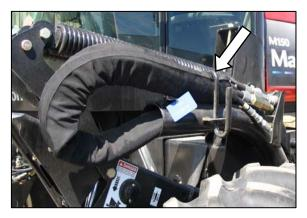
r. Rotate hook, and re-engage in bracket.
