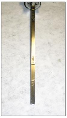
n. Check hydraulic oil level in reservoir. necessary, add SAE15W-40 oil.
