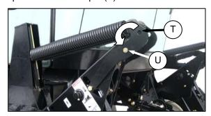
Remove pin from storage position (T) in linkage, and insert in hole (U) to engage float springs. Secure with hairpin.
