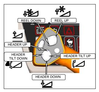
e. Adjust the position of the center-link cylinder with the REEL UP and REEL DOWN switches, and HEADER TILT switches on the GSL to position the hook above the header attachment pin.
