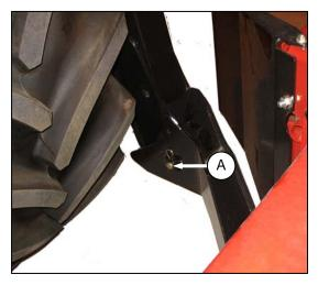
i. Install pin (A) through each boot and foot, and secure with hairpin.
