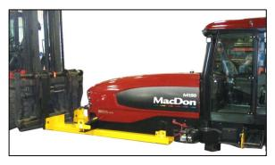
a. Approach windrower from aft end, and slide forks fully into shipping support channels.
