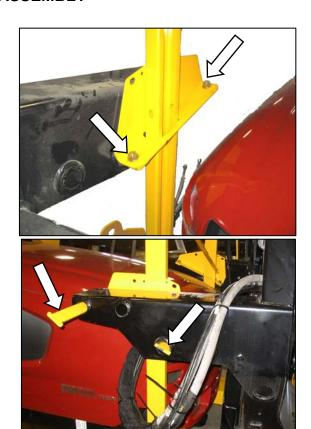
d. Remove two bolts near top of leg, and remove bars from leg.
