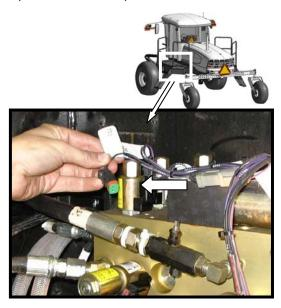
g. Disconnect brake engage solenoid connector (P-V3) at valve block on LH side of windrower.
