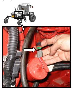
i. Disconnect electrical connection at fuel pump on right side of engine.
