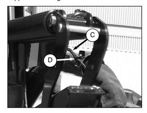
p. Attach harness (C) to hose support with hose clip (D).
