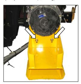
c. Remove two bolts at lower support channel.
