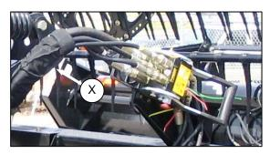
Connect reel hydraulics (X) at RH side of windrower. Refer to the Draper Header Operator's Manual.
