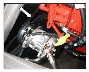
a. Tension on A/C compressor belt should be such that a force of 8–12 lbf (35–55 N) deflects the belt 3/16 inch (5 mm) at mid-span.
