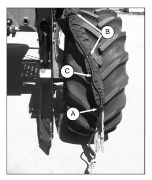
p. Secure harness (C) to hose bundle with strap (A) and new plastic cable ties (B). Ensure harness is clear of pinch and friction points.
