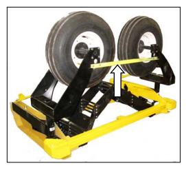
d. Remove tie bar between the two caster wheels.
