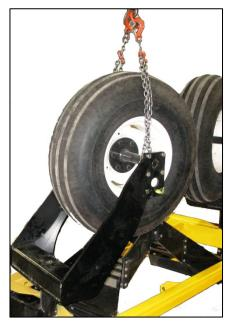
f. Attach a chain to RH caster, and support caster with lifting device.
