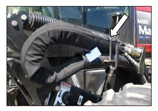
s. Rotate hook, and re-engage in bracket.
