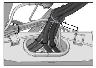
n. Insert four traction drive hoses into slots in block as shown, and reinstall clamp.
