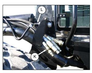
Connect header drive hydraulics (K) and electrical harness (L) to header. Refer to your Auger Header Unloading and Assembly Instructions.
