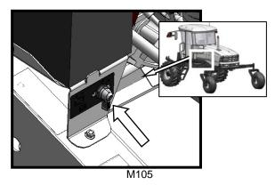
**M105:** A battery main disconnect switch is located on the LH frame rail on the battery tray, and can be accessed by raising the engine compartment hood.
