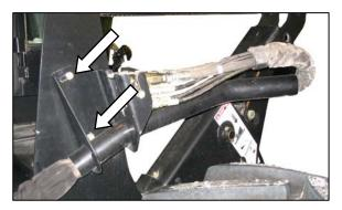
s. Attach reel hose support tube to the RH reel leg with two 3/8 in. x 1.0 carriage bolts and nuts.
