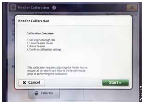
Figure 8.320: John Deere S7 Display – Header Calibration
