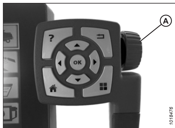
Figure 8.198: Adjustment Wheel on Right Side of Tyton Terminal
