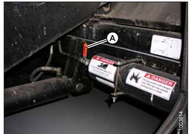
Figure 7.180: Combine Accumulator ON/OFF Switch A - Accumulator Lever (Off Position)
