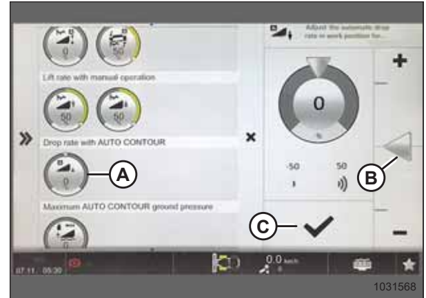
Figure 7.166: Drop Rate with Auto Contour Page
