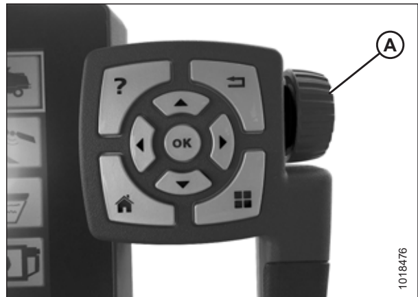
Figure 7.220: Adjustment Wheel on Right Side of Tyton Terminal
