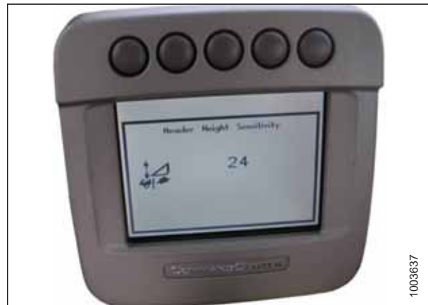
Figure 7.234: John Deere Combine Display
