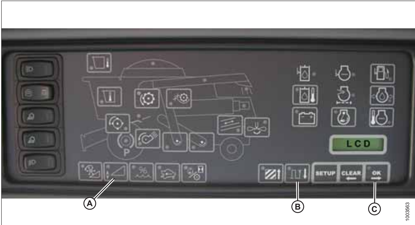
Figure 7.176: Combine Heads-Up Display
