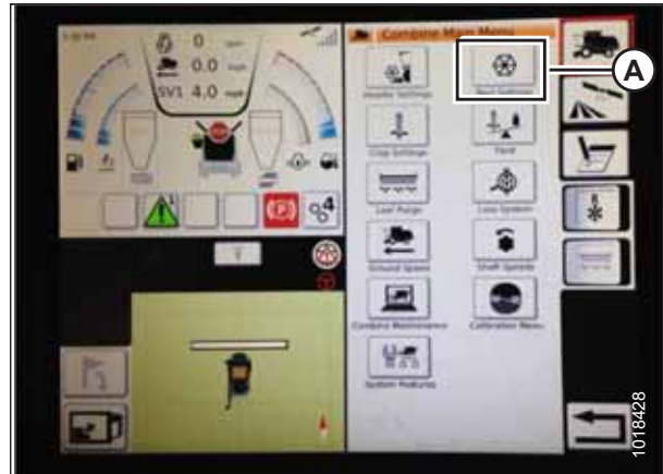
Figure 7.197: Reel Settings on Combine Main Menu
