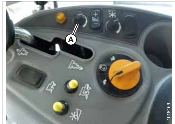
Figure 7.104: Height Adjustment Knob on the Combine Control Console
