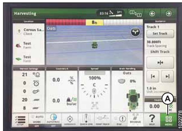
Figure 7.300: John Deere S7 Display – Harvesting Page
