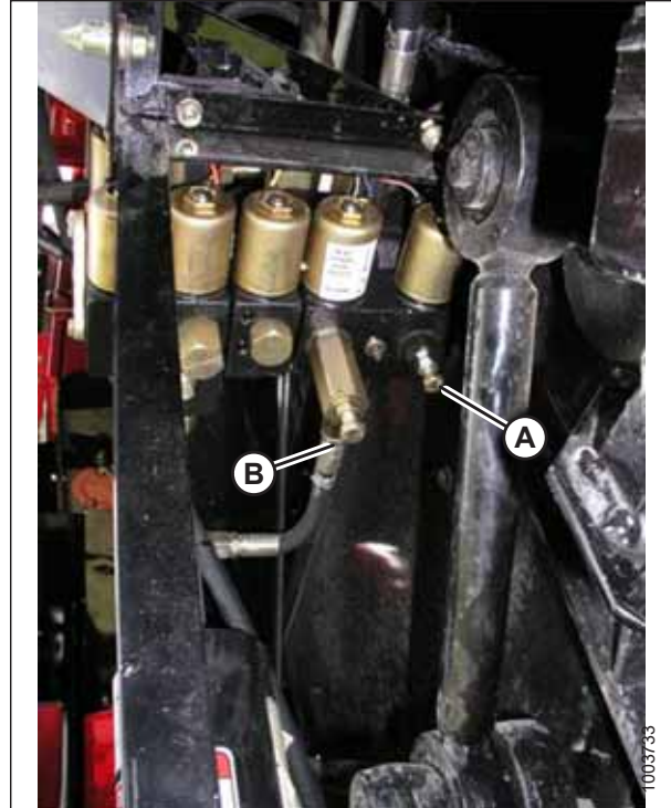
Figure 7.181: Header Raise and Lower Adjustable Restrictors
