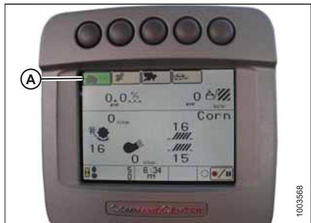
Figure 7.224: John Deere Combine Display
