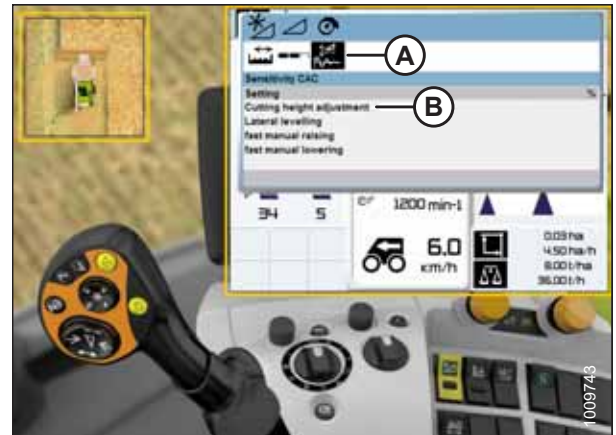
Figure 7.139: CLAAS Combine Display
