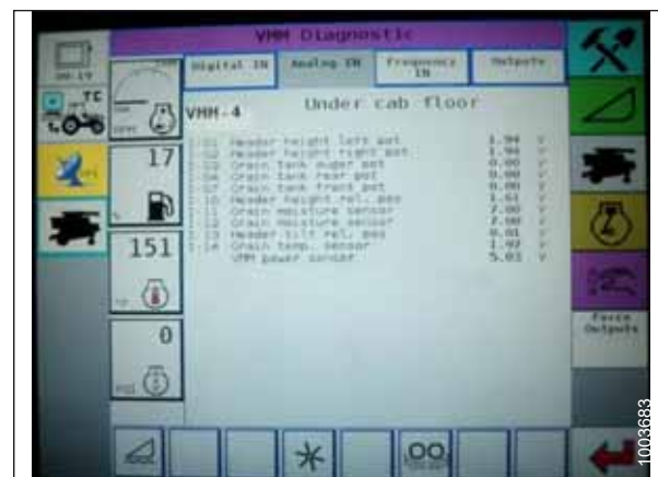
Figure 7.97: Challenger Combine Display
