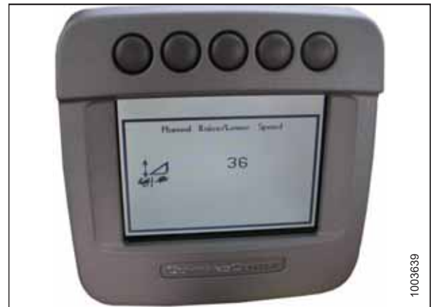
Figure 7.236: John Deere Combine Display
