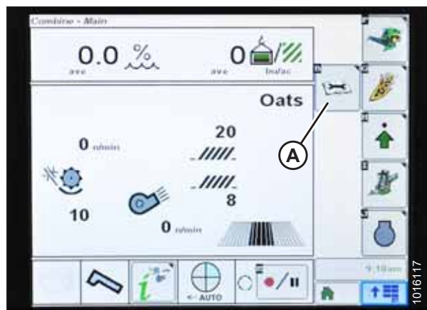
Figure 7.266: John Deere Combine Display
