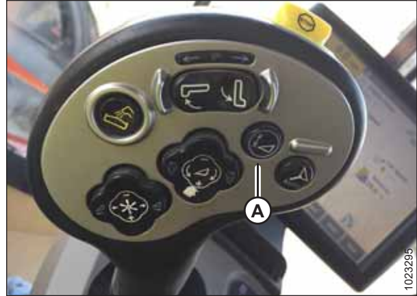
Figure 7.59: Case Combine Control Handle
