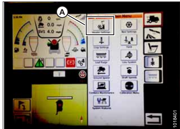
Figure 7.189: Header Settings in Combine Main Menu
