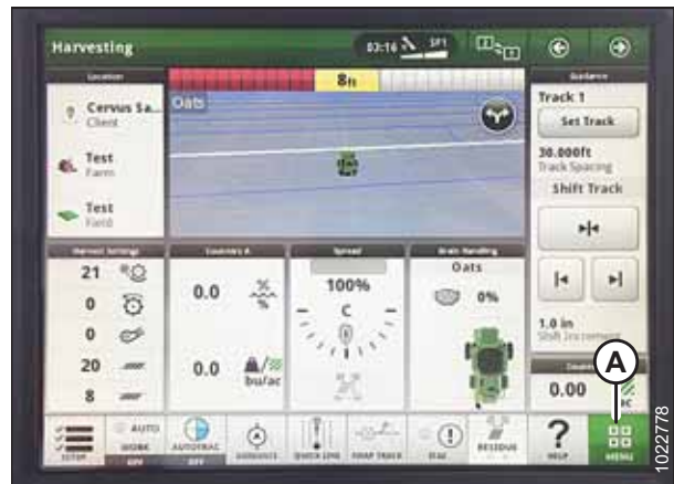
Figure 7.307: John Deere S7 Display – Harvesting Page
