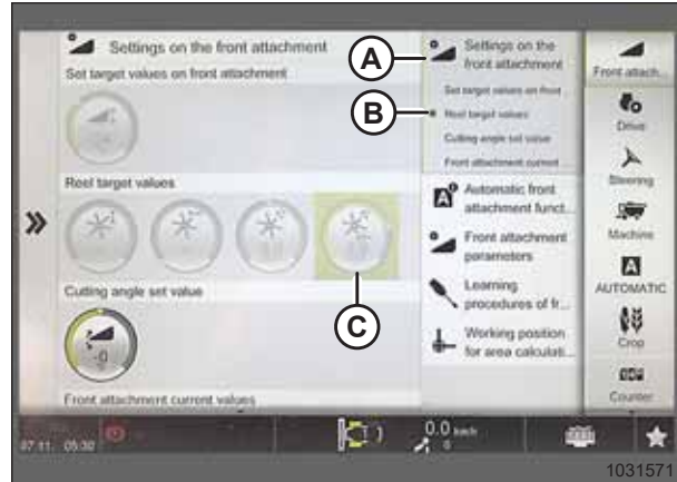
Figure 7.168: Settings on Front Attachment Page
