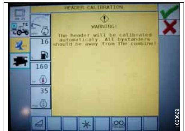
Figure 7.102: Challenger Combine Display
