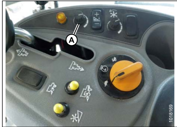
Figure 6.61: Height Adjustment Knob on the Combine Control Console
