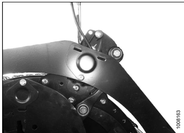
Figure 4.113: Right Reel with Cam Arms Attached
