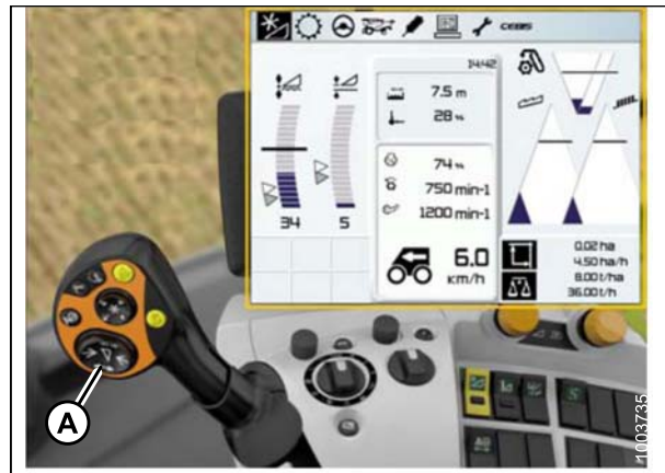
Figure 6.197: CLAAS Combine Display, Console, and Joystick Lever
