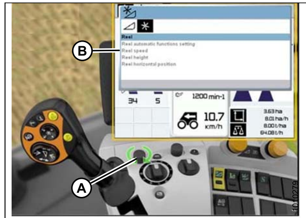
Figure 6.202: CLAAS Combine Display, Console, and Joystick Lever
