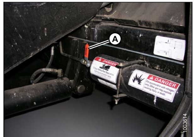
Figure 6.73: Combine Accumulator On/Off Switch
