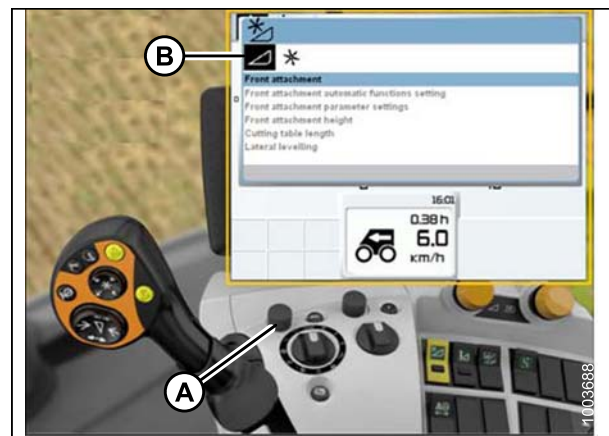
Figure 6.192: CLAAS Combine Display, Console, and Joystick Lever
