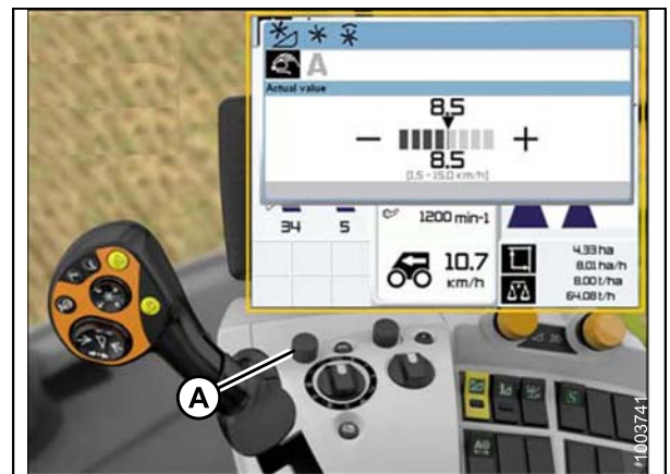
Figure 6.204: CLAAS Combine Display, Console, and Joystick Lever
