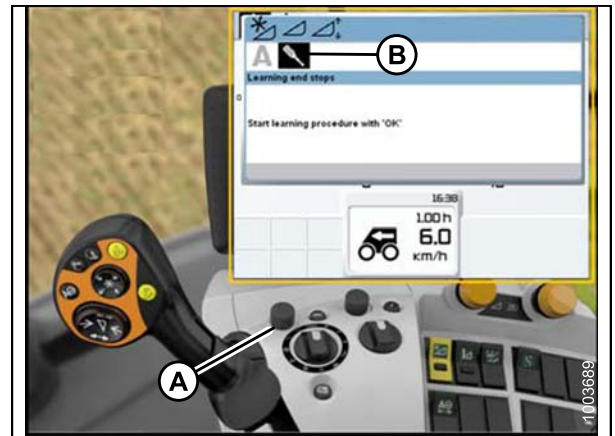
Figure 6.194: CLAAS Combine Display, Console, and Joystick Lever
