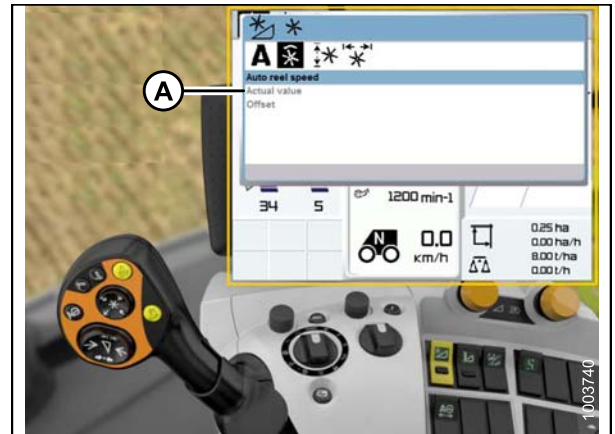
Figure 6.203: CLAAS Combine Display, Console, and Joystick Lever
