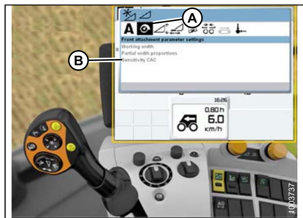
Figure 6.199: CLAAS Combine Display, Console, and Joystick Lever
