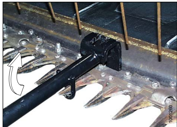
Figure 8.7: Guard Tips – Upward Adjustment
