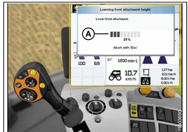
Figure 6.195: CLAAS Combine Display, Console, and Joystick Lever
