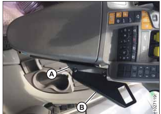
Figure 5.64: Top View of Armrest Showing Supports Installed in Preferred Location
