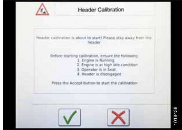
Figure 7.243: Header Calibration Warning
