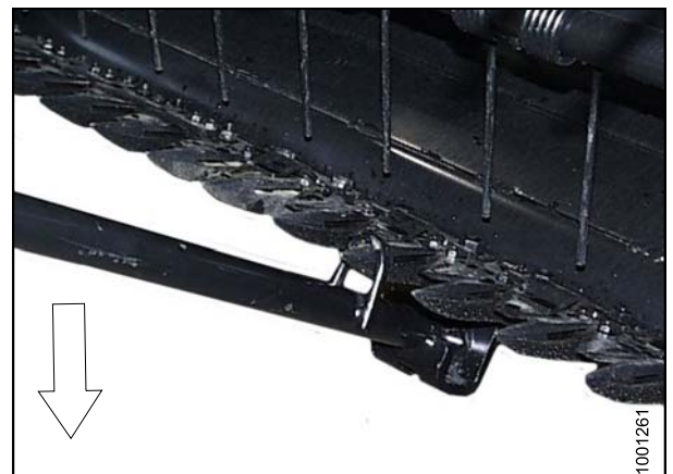
Figure 8.27: Guard Tips – Downward Adjustment
