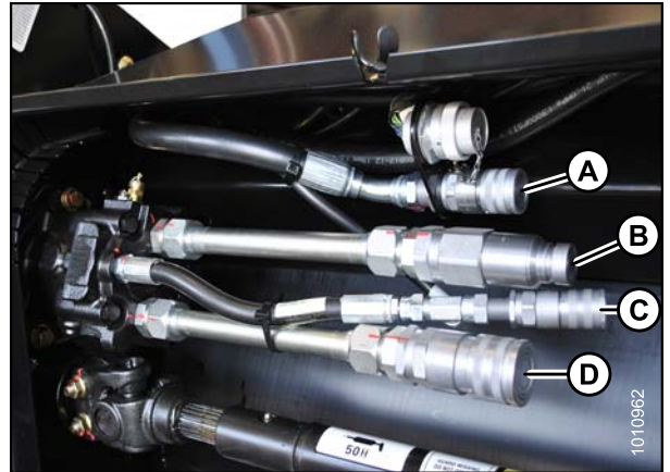
Figure 6.106: Hose Connections on Standard Header – 18 Ft. Header Shown
