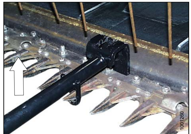
Figure 8.26: Guard Tips – Upward Adjustment
