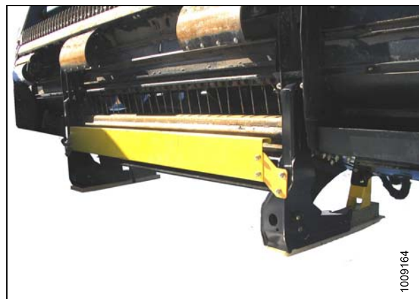
Figure 5.3: Underside of Header in Shipping Configuration
