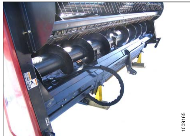
Figure 5.2: Topside of Header in Shipping Configuration
