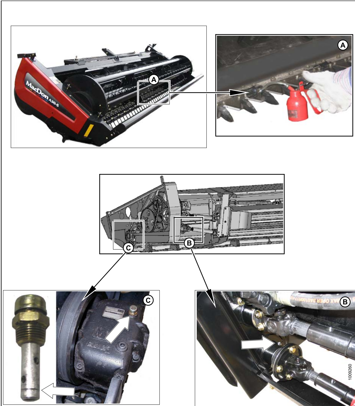
Figure 7.6: Oiling (SAE 30 Oil)
