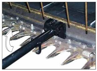
Figure 4.28: Guard Tip – Upward Adjustment
