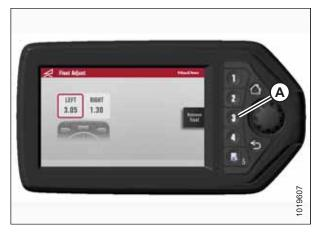
Figure 3.122: HPT Display - Adjusting Float
