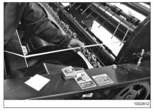
Figure 3.100: Measuring Reel Fore-Aft Offset
