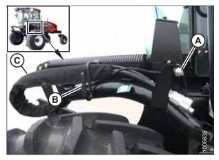
Figure 3.59: Support Bracket and Hose Bundle
