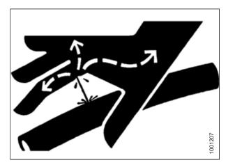
Figure 1.12: Hydraulic Pressure Hazard
