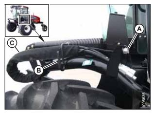
Figure 3.45: Support Bracket and Hose Bundle
