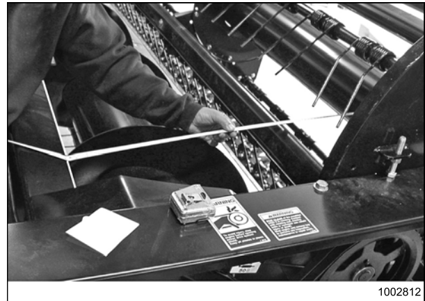
Figure 3.88: Measuring Reel Fore-Aft Offset
