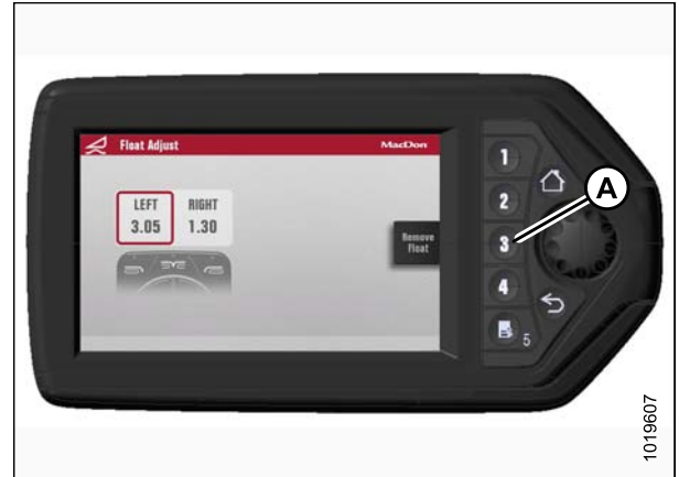
Figure 3.110: HPT Display – Adjusting Float
