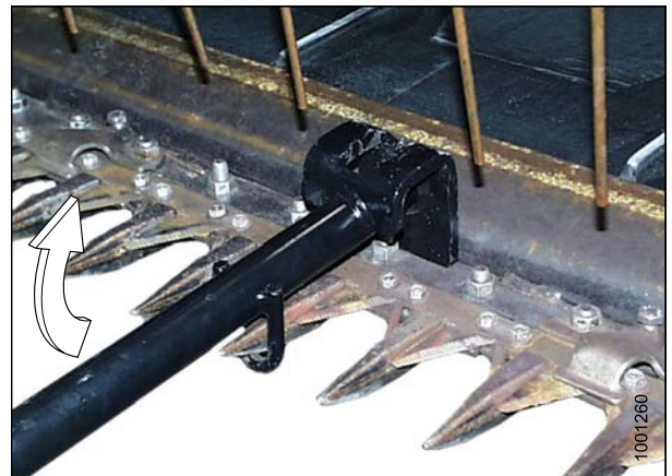
Figure 4.26: Guard Tip – Upward Adjustment
