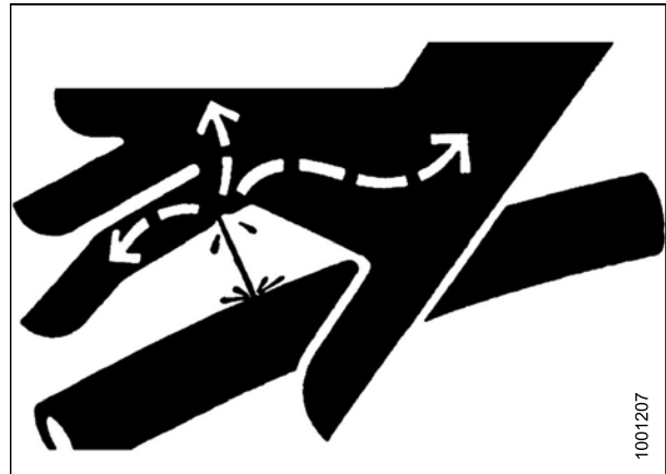
Figure 1.12: Hydraulic Pressure Hazard
