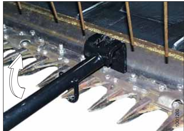
Figure 5.44: Guard Tips – Upward Adjustment
