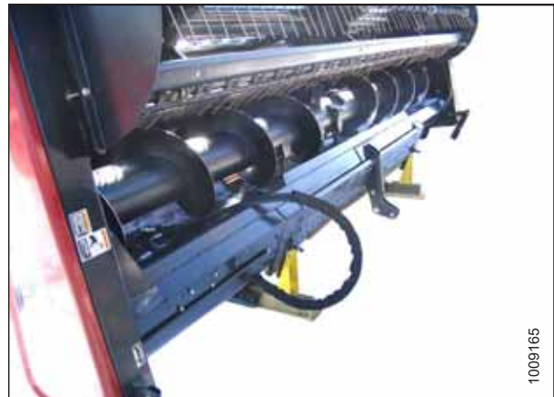
Figure 2.2: Topside of Header in Shipping Configuration
