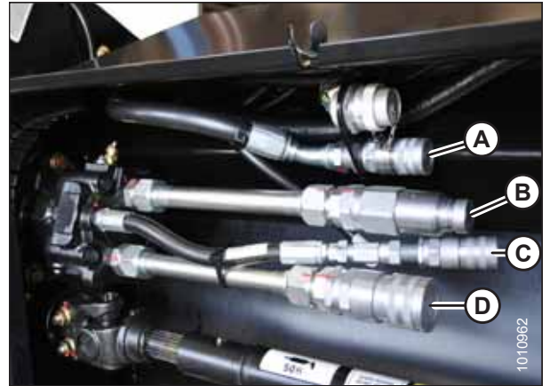
Figure 3.52: A40D Hose Connections – 5.4 m (18 ft.) Header Shown
