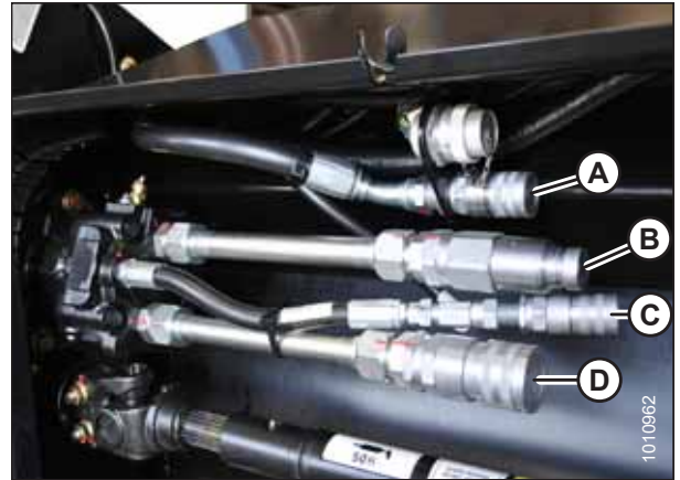
Figure 3.82: A40D Hose Connections – 5.4 m (18 ft.) Header Shown
