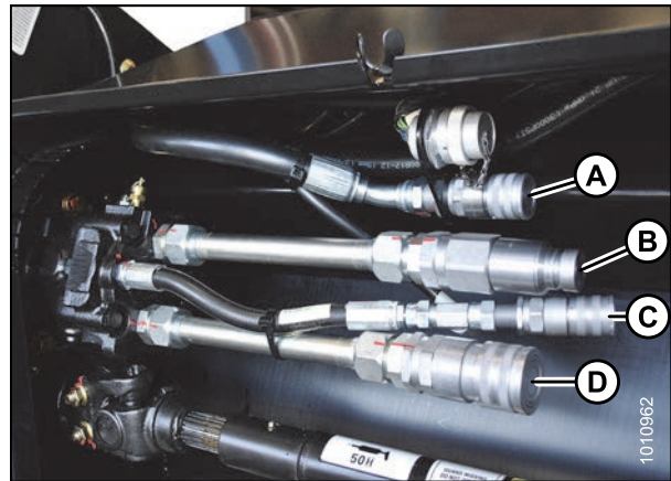
Figure 3.116: Hose Connections on Standard Header – 18-Ft. Header Shown
