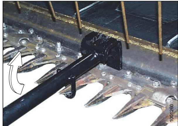
Figure 5.26: Guard Tips – Upward Adjustment
