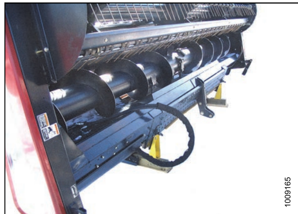
Figure 2.2: Topside of Header in Shipping Configuration
