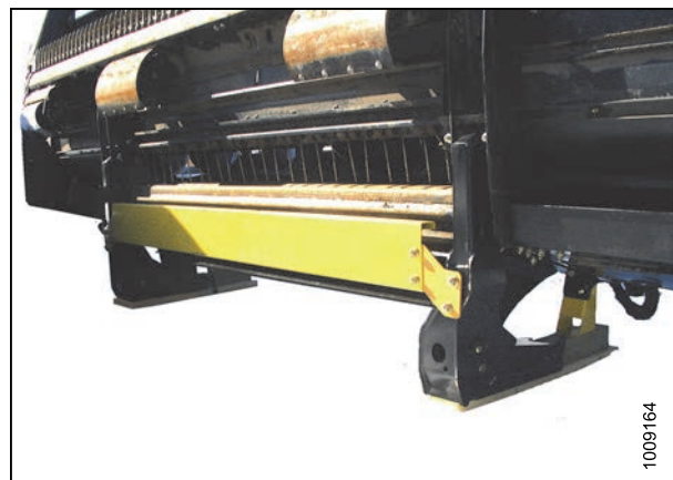
Figure 2.3: Underside of Header in Shipping Configuration
