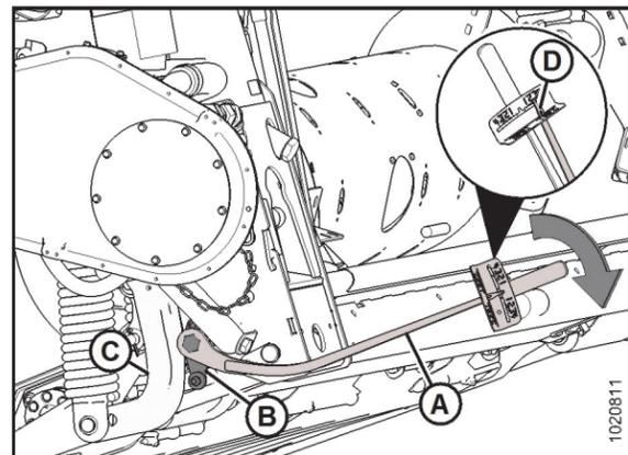
Figure 6: Checking Float – Left Side Shown
