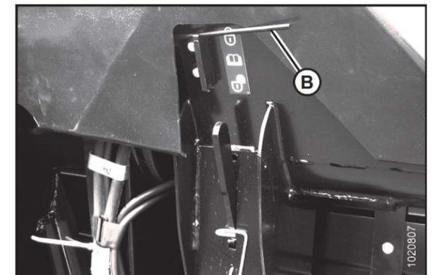
Figure 2: Wing Lock Spring Handle in Locked Position
