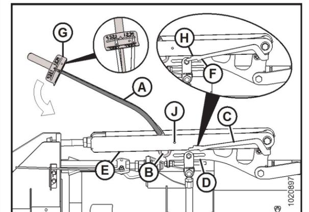
Figure 9: Wing Balance Linkage, Wings Set too Heavy – Left Side, Right Opposite
