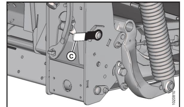
Figure 3: Float Unlocked - Right Side Shown
