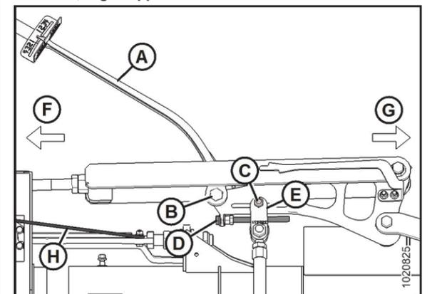
Figure 10: Wing Balance Linkage – Left Side Shown
