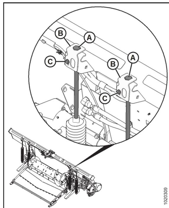
Figure 7: Float Adjustment Bolts – Left Side Shown
