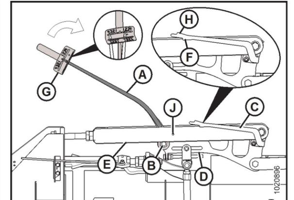
Figure 8: Wing Balance Linkage, Wings Set too Light – Left Side, Right Opposite
