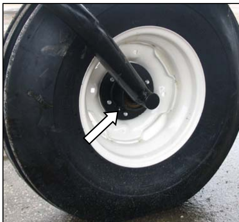
FORMED CASTER WHEEL BEARING 1 PLACE (BOTH WHEELS)
