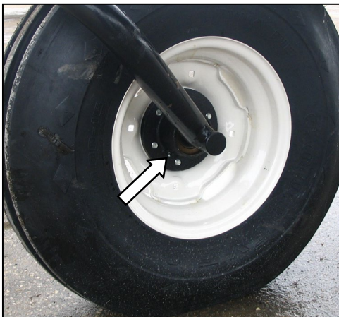
FORMED CASTER WHEEL BEARING 1 PLACE (BOTH WHEELS)
