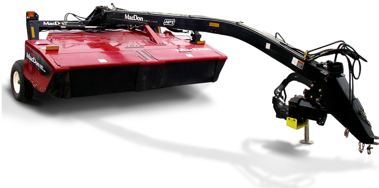
R80 PULL-TYPE ROTARY DISC MOWER CONDITIONER
