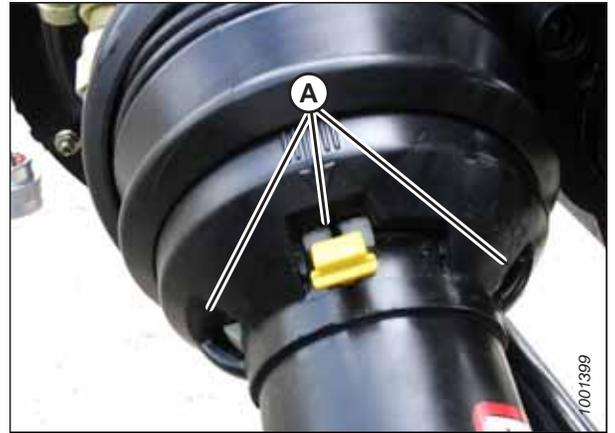
Figure 5.46: Protection de transmission
