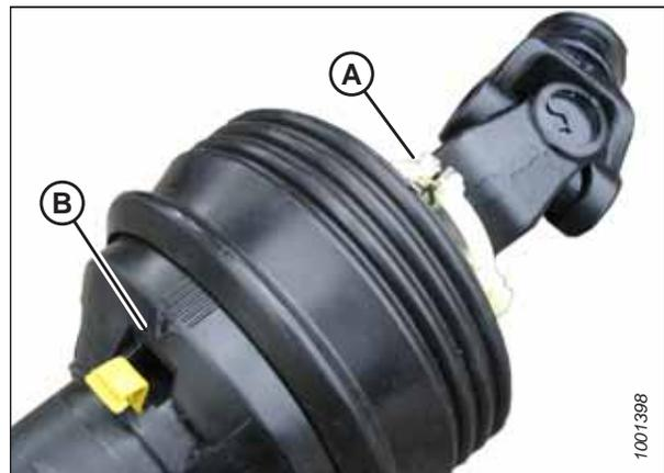
Figure 5.45: Protection de transmission
