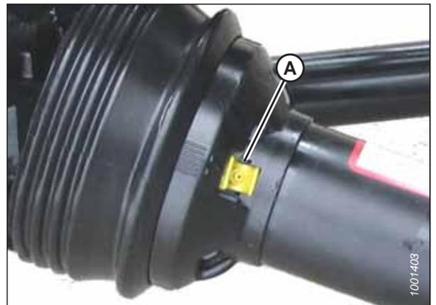
Figure 5.48: Protection de transmission
