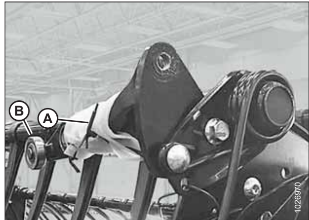
Figure 4.30: Cam Arm in Shipping Position
