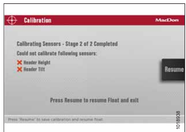
Figure 6.70: Sample of Failed Calibration Display Message
