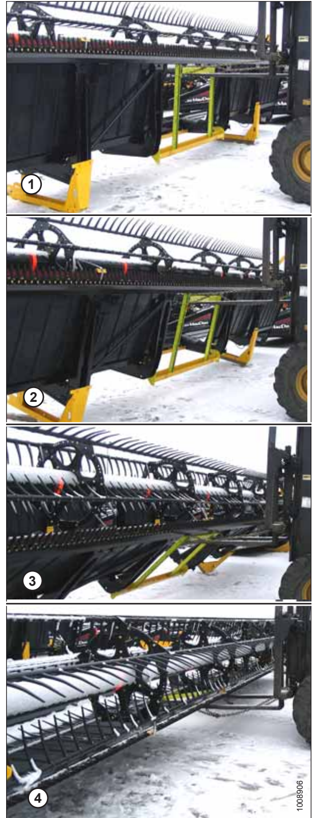
Figure 2.10: Lowering the Header
