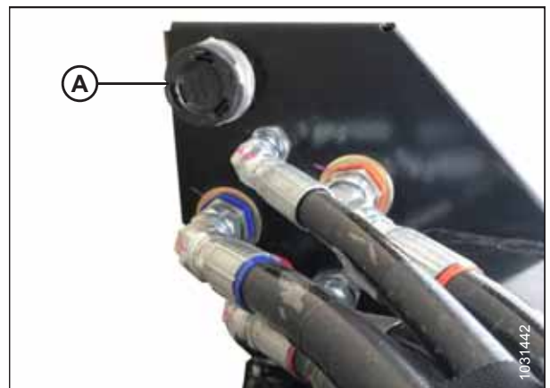
Figure 5.11: Electrical Connector on Header for Hydraulic Hose Management System
