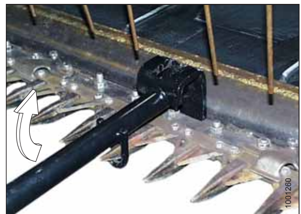
Figure 8.2: Straightening Tool – Upward Adjustment
