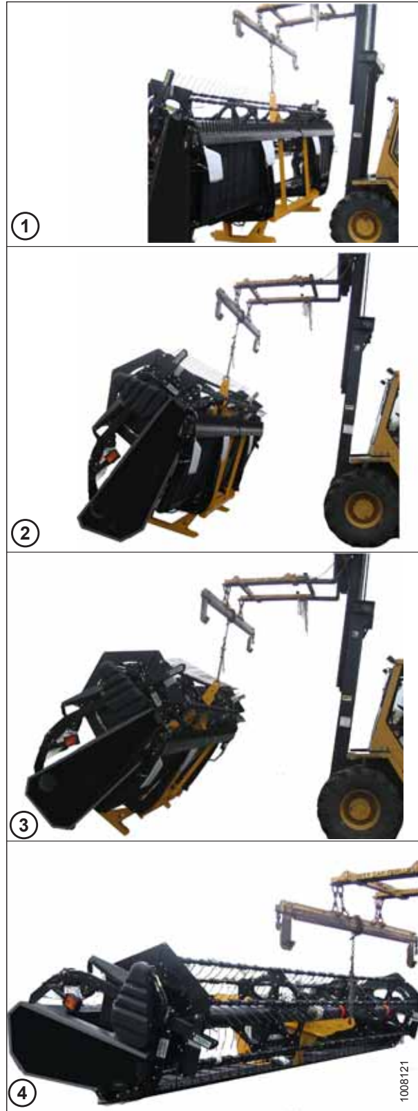
Figure 2.5: Lowering the Header
