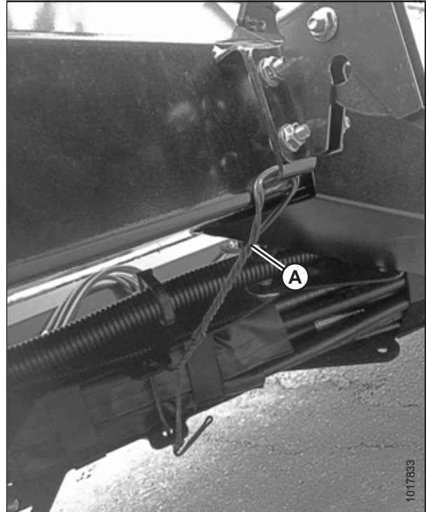
Figure 5.7: Hydraulic Hose Management System in Shipping Position – D140XL and D145XL Headers
