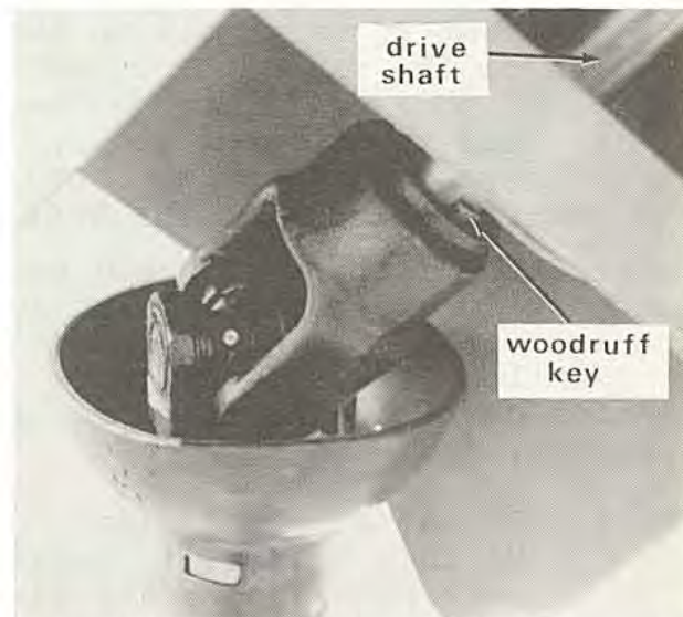
P.T.O. SHAFT- partially installed
