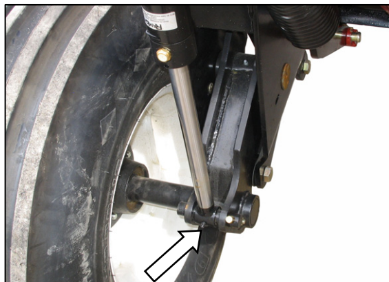
CYLINDER PIVOT 1 PLC
