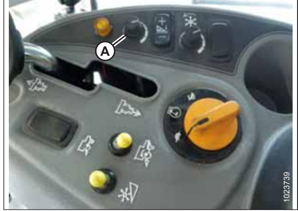
Figure 6.82: Height Adjustment Knob on Combine Control Console
