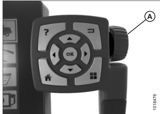
Figure 6.35: Adjustment Wheel on Right of Tyton Terminal
