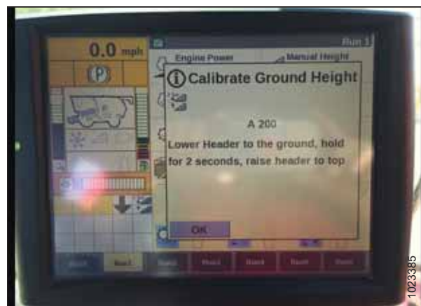
Figure 6.45: Calibrating Auto Header Height
