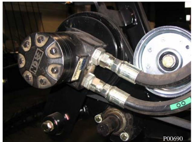
**Hydraulic Motor Installed**
