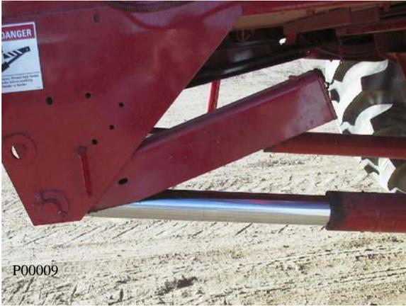
**Disengaged Feeder House Lock**
