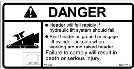
1. Header Crushing Hazard - 184398
