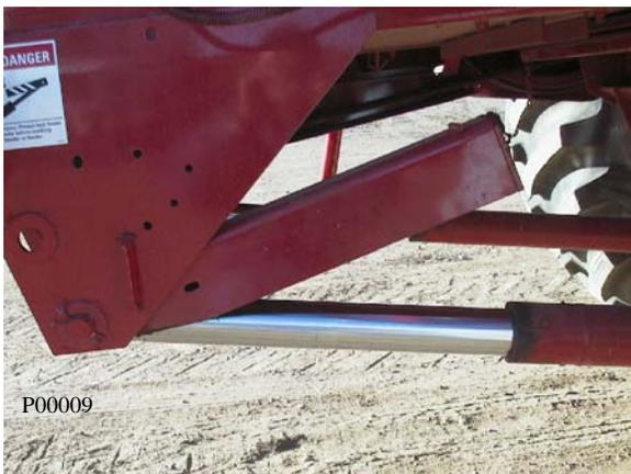
**Feeder house Lock Disengaged**
