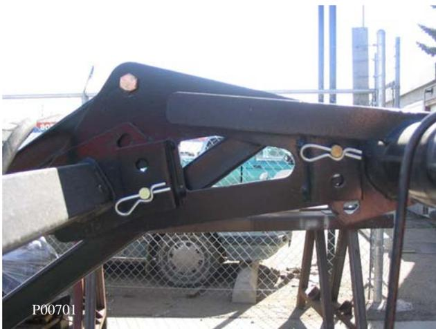
**Hold-down Clevis and Hitch Pins**
