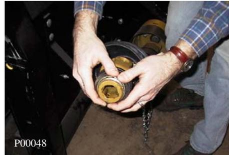
**Drive Shaft to Header Installation**
