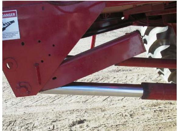
**Disengaged Feeder House Lock**
