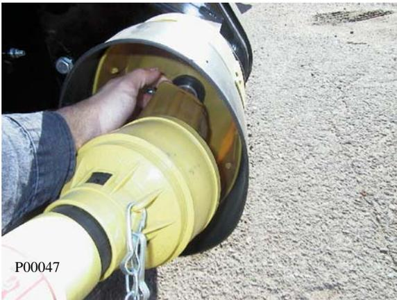
**Drive Shaft to Header Installation**
