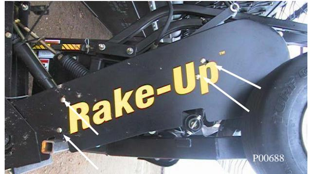
**Rake-Up Drive Shield Removal**
