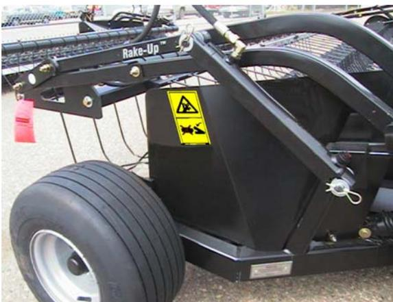
**Pinch Point Located on LH Idler Rotor
