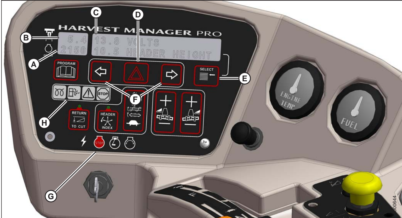
Figure 3.68: Cab Display Module (CDM) Engine and Windrower Functions
