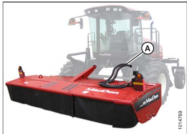
Figure 4.217: Header Drive Hydraulics
