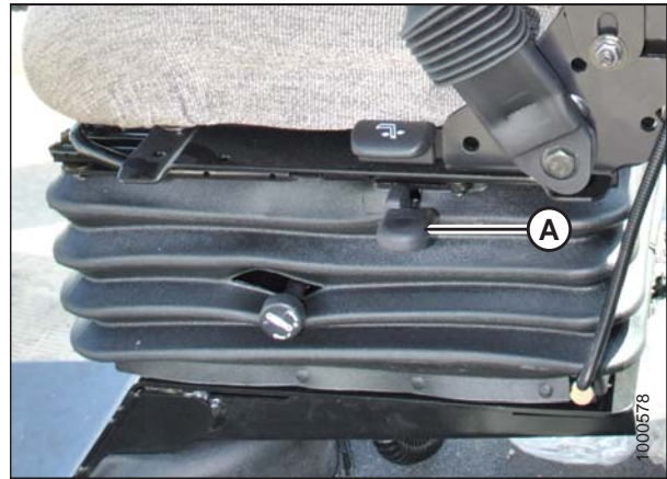
Figure 3.8: Fore-Aft Isolator Lock
