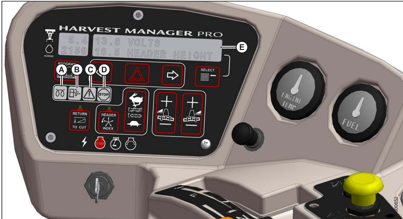
Figure 3.71: CDM Engine Warning Lights
