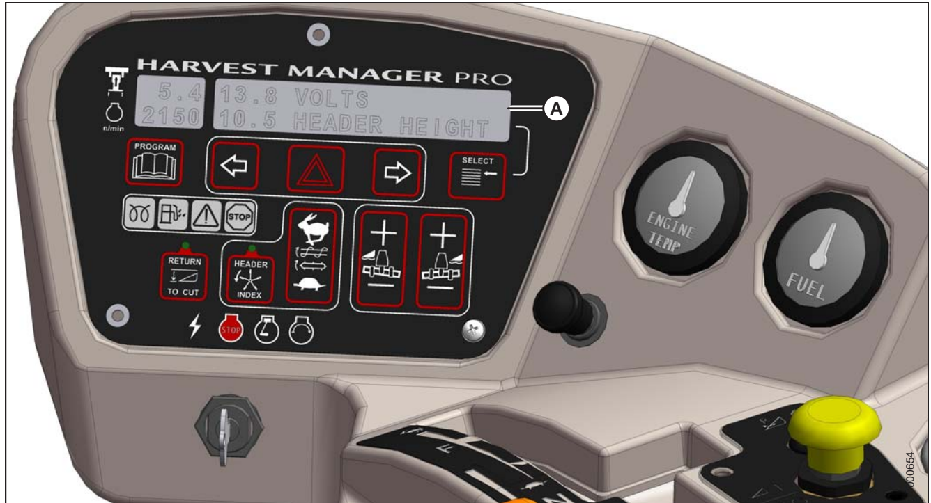
Figure 3.72: CDM Display Warnings and Alarms
