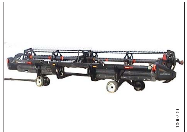
Figure 4.39: Header in Transport Mode
