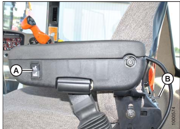
Figure 3.5: Seat Suspension and Height
