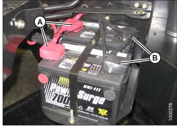
Figure 5.116: Battery Terminal Location
