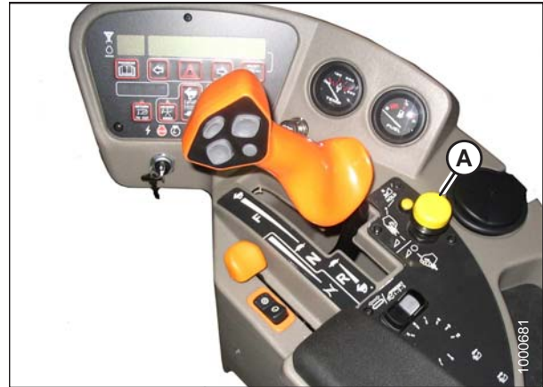
Figure 4.32: Header Drive Switch
