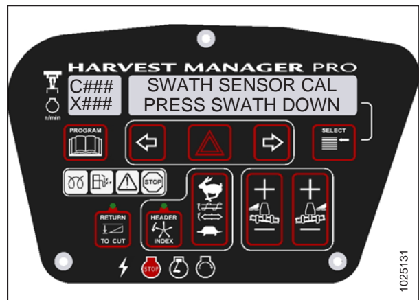
Figure 3.164: Swath Compressor Sensor Calibration
