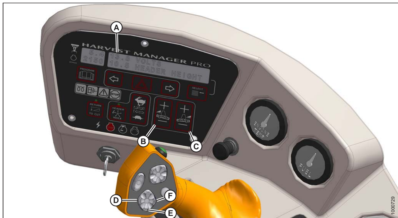
Figure 4.67: Cab Display Module (CDM) Float Adjustment
