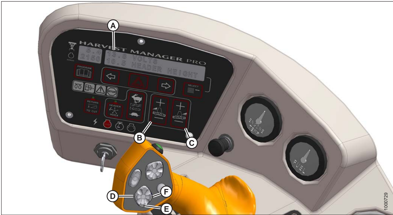
Figure 4.71: Cab Display Module (CDM) Float Adjustment
