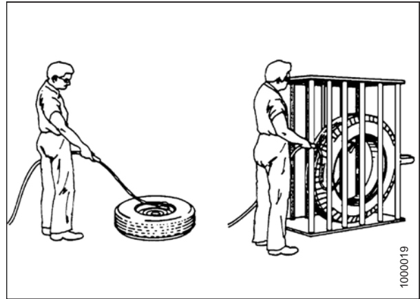
Figure 5.214: Safely Filling a Tire with Air
