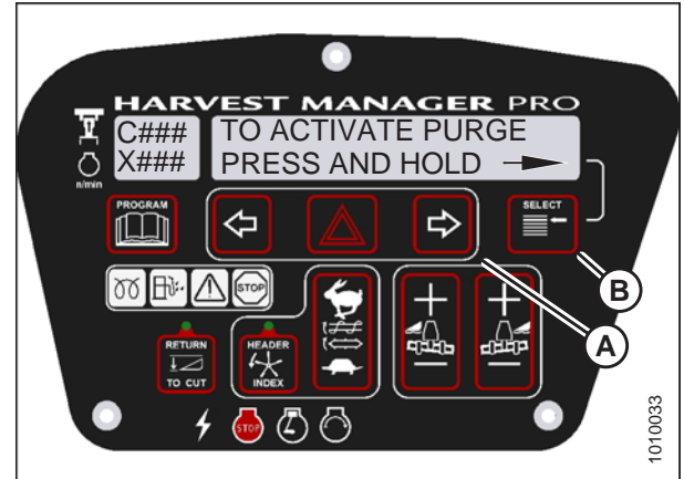
Figure 3.219: M205 Hydraulic Purge
