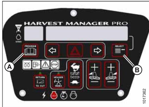
Figure 3.115: Cab Display Module (CDM)
