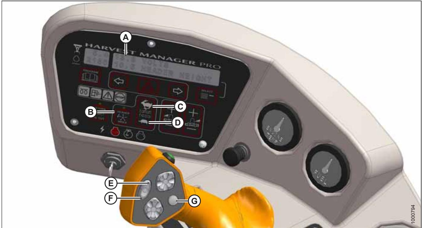
Figure 4.300: Operator Console
