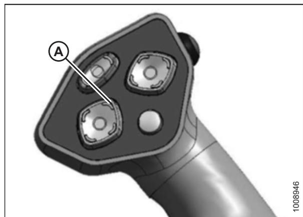
Figure 4.232: Ground Speed Lever
