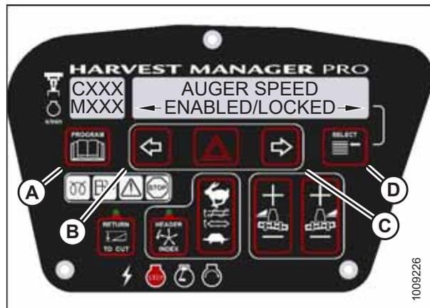
Figure 3.130: Auger Control Lock
