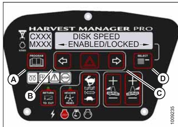
Figure 3.136: Disc Speed Control Lock
