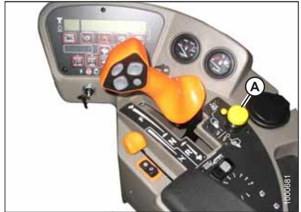
Figure 4.32: Header Drive Switch
