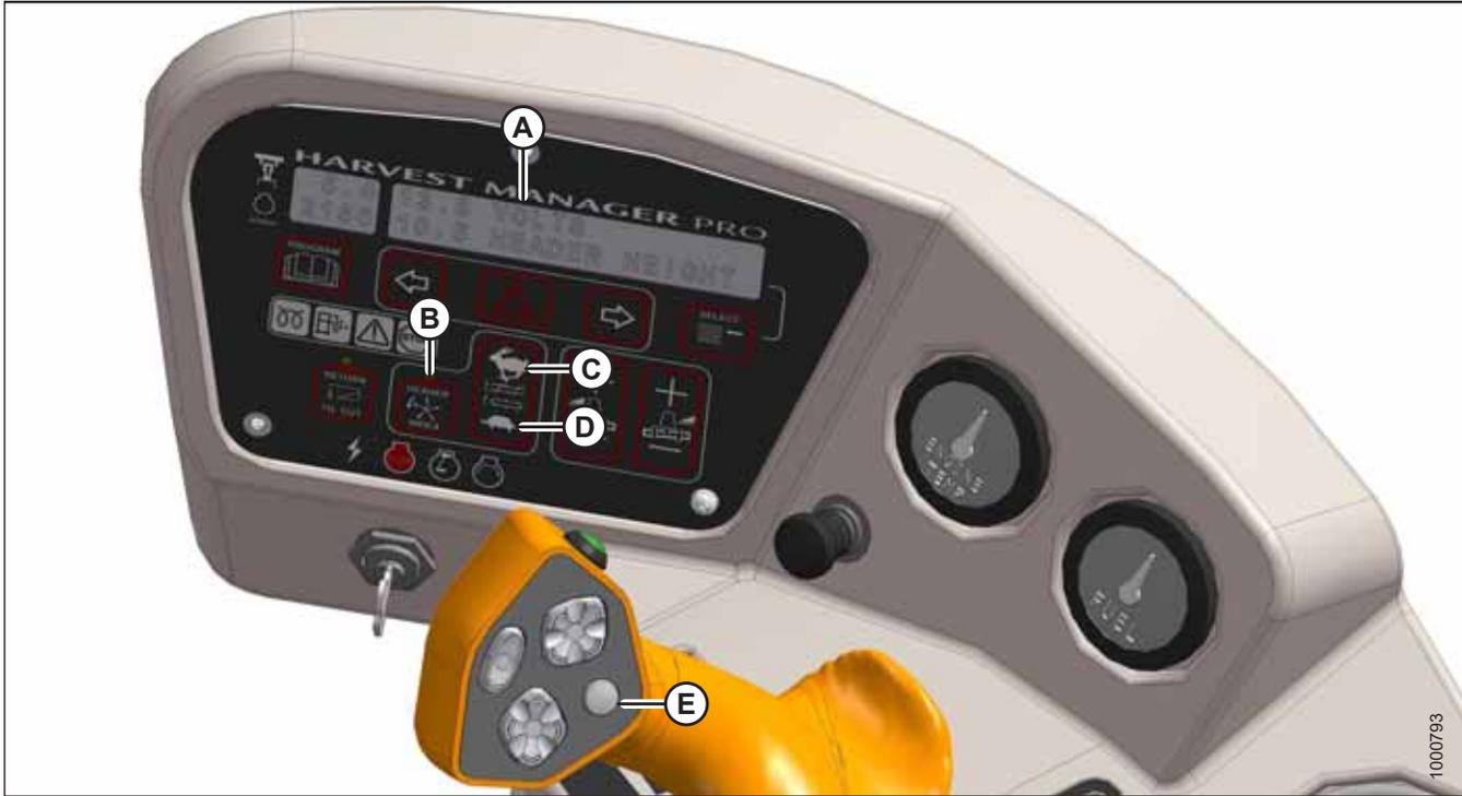
Figure 4.292: Operator Console
