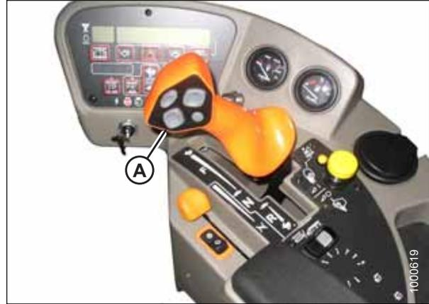
Figure 5.21: Operator Console
