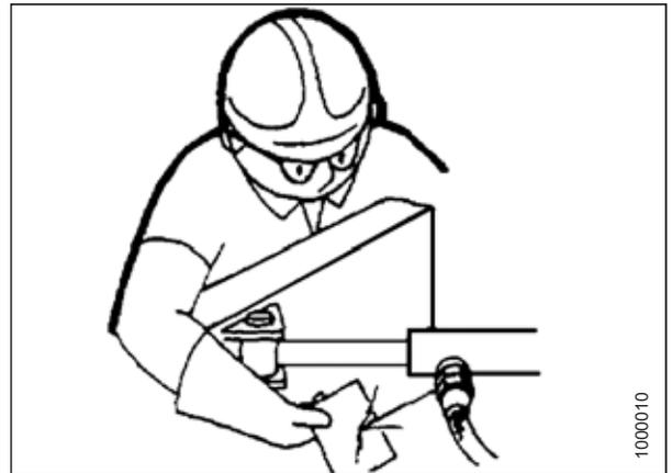
Figure 5.192: Checking Hydraulic Leaks
