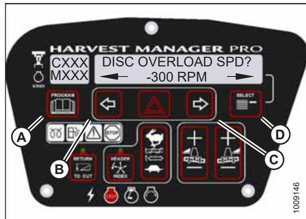
Figure 3.83: Disc Overload Speed
