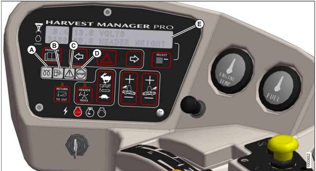
Figure 3.60: CDM Engine Warning Lights
