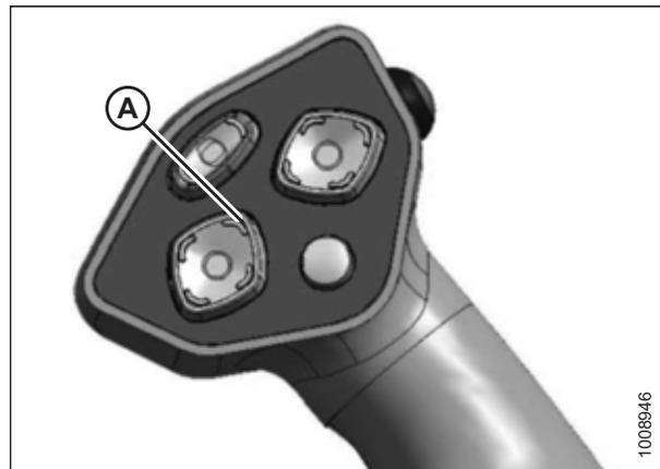
Figure 4.216: Ground Speed Lever
