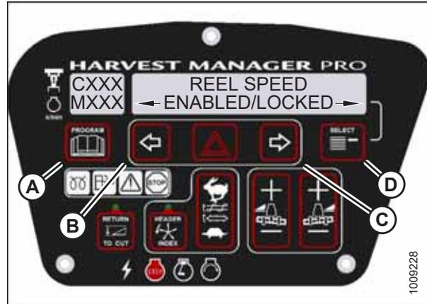
Figure 3.139: Reel Speed Control Lock
