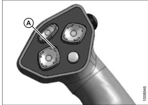
Figure 4.144: Ground Speed Lever (GSL)
