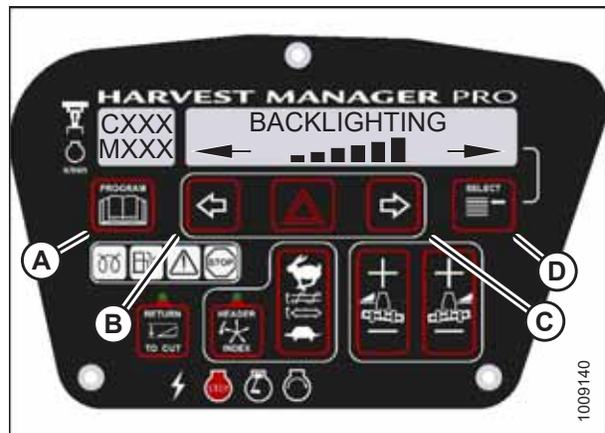
Figure 3.74: Display Backlighting Setting
