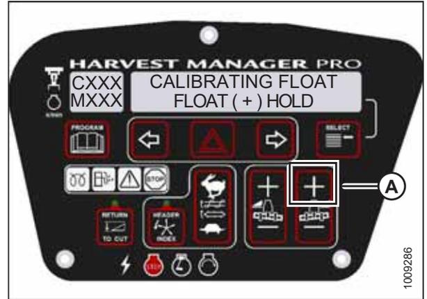
Figure 3.155: Positive Header Float Display
