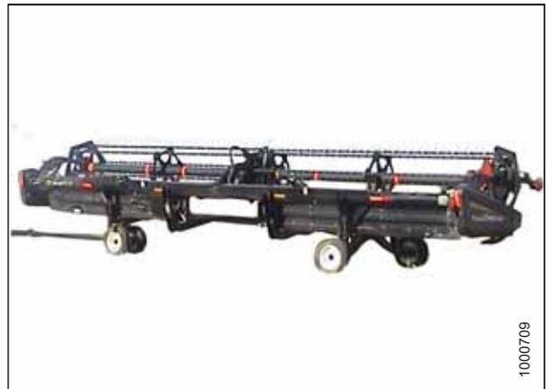
Figure 4.40: Header in Transport Mode
