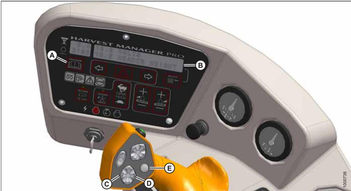
Figure 4.87: Operator Console
