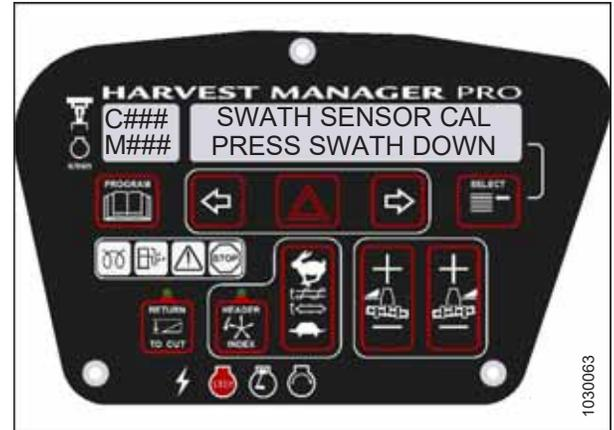
Figure 3.160: Swath Compressor Sensor Calibration
