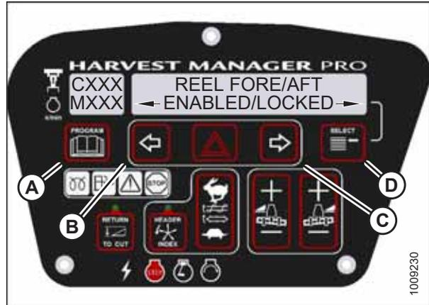
Figure 3.124: M155 Reel Fore-Aft Control Lock
