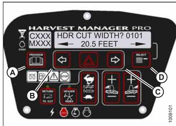
Figure 3.101: Header Cut Width
