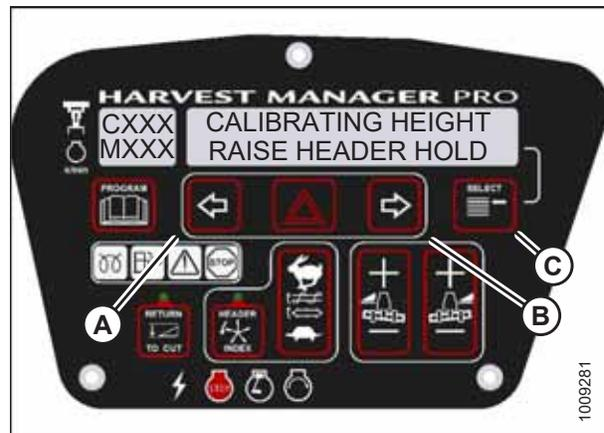
Figure 3.145: Header Height Calibration
