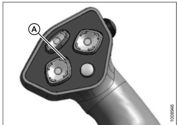
Figure 4.154: Ground Speed Lever
