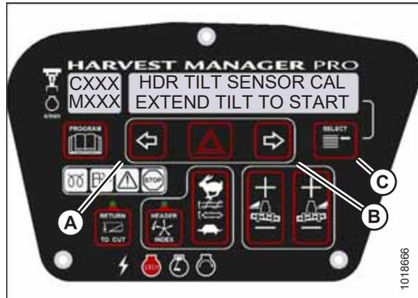
Figure 3.149: Header Tilt Calibration
