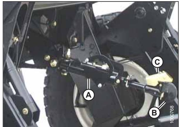
Figure 4.213: Hydraulic Center-Link
