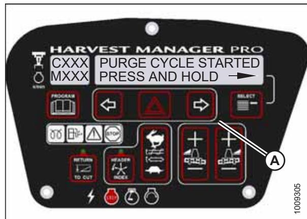
Figure 3.216: Hydraulic Purge Cycle
