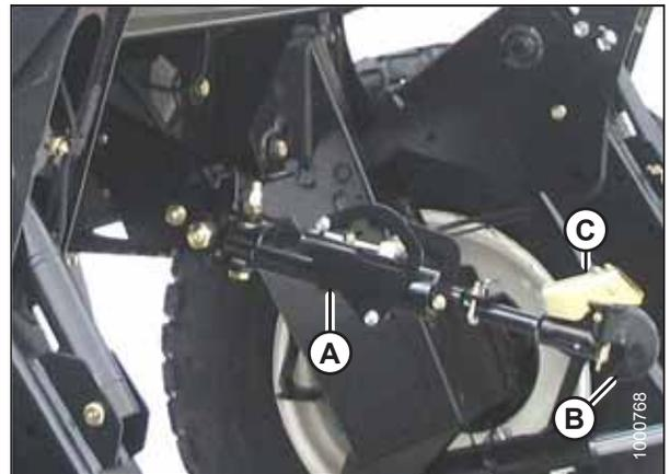
Figure 4.271: Hydraulic Center-Link
