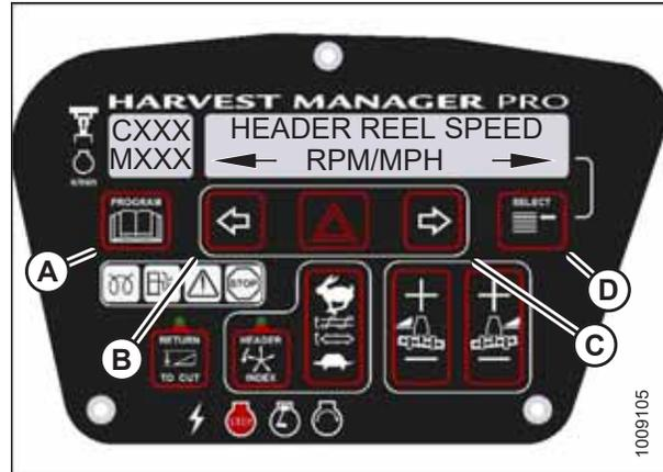
Figure 3.109: Reel Speed Display
