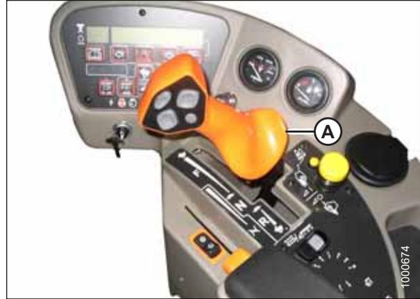
Figure 4.26: Operator Console
