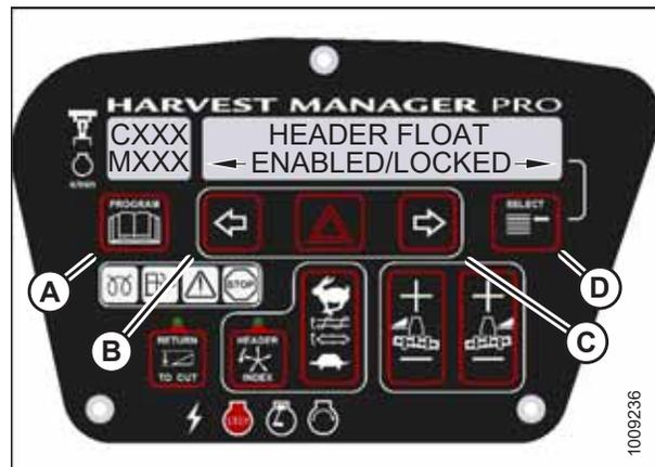
Figure 3.121: Header Float Control Lock
