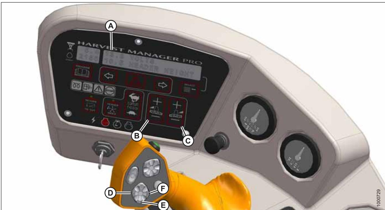
Figure 4.75: Cab Display Module (CDM) Float Adjustment
