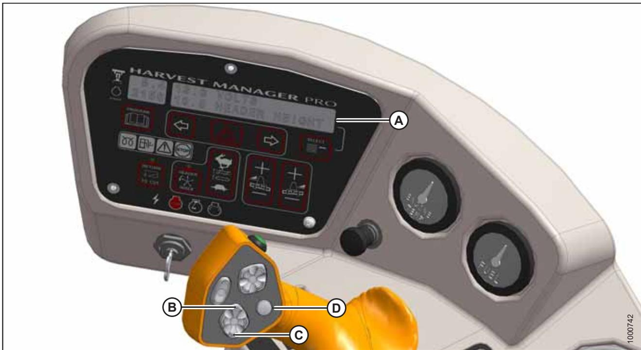
The cab display module (CDM) indicates header height with a reading on the DISPLAY (A) lower line between 00.0 and 10.0, with 00.0 being on the ground.
