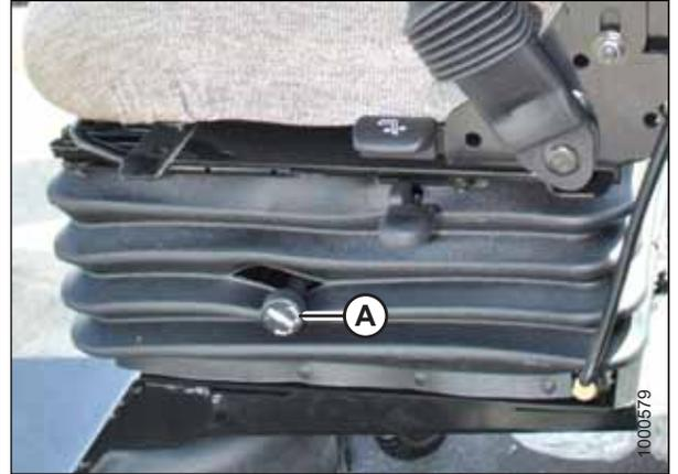
Figure 3.6: Vertical Dampener
