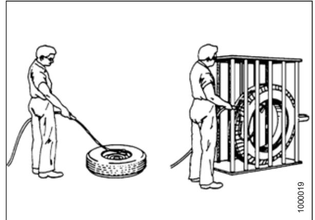
Figure 5.210: Safely Filling a Tire with Air
