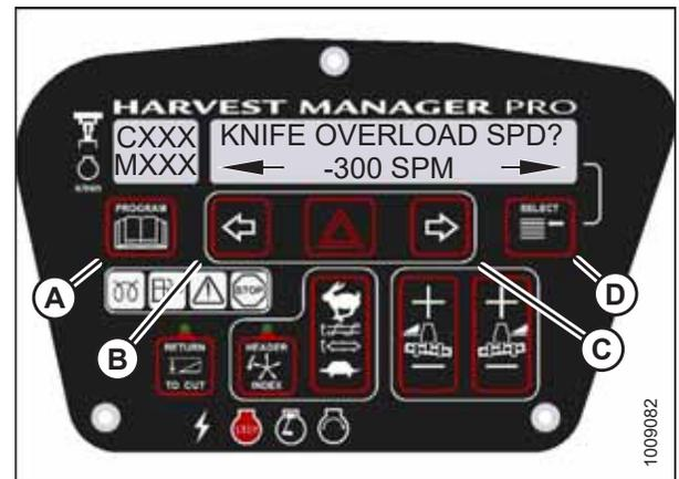
Figure 3.81: Knife Overload Speed
