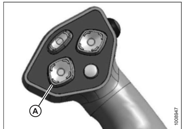
Figure 4.251: Ground Speed Lever
