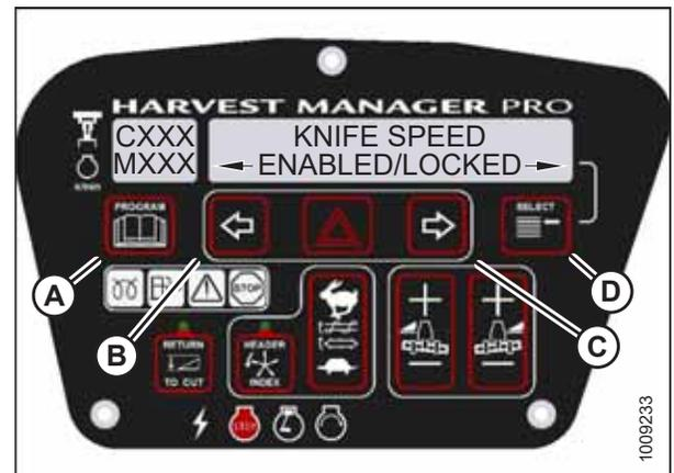
Figure 3.133: Knife Speed Control Lock
