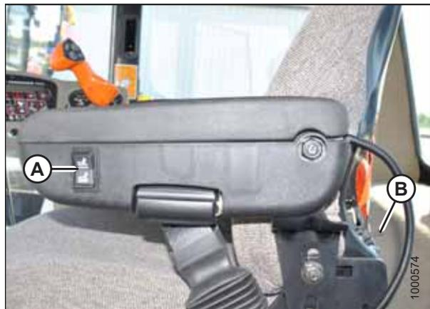
Figure 3.5: Seat Suspension and Height
