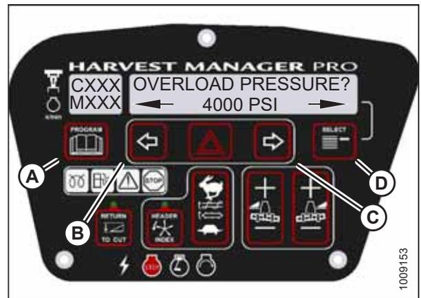
Figure 3.85: Hydraulic Overload Pressure
