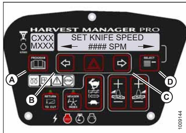
Figure 3.79: Knife Speed Setting
