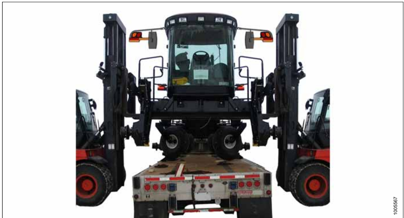
Figure 2.1: Two-Forklift Unloading Method
