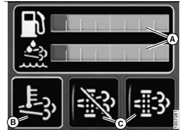
Figure 4: Diesel Exhaust Fluid (DEF) Display Monitor
