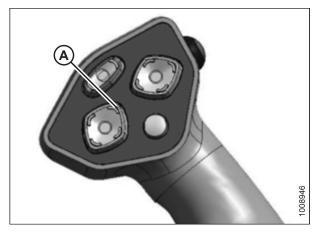
Figure 4.122: Ground Speed Lever
