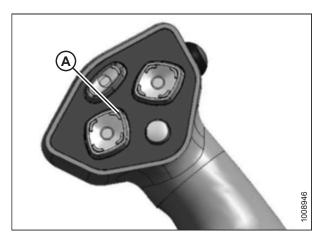
Figure 4.227: Ground Speed Lever
