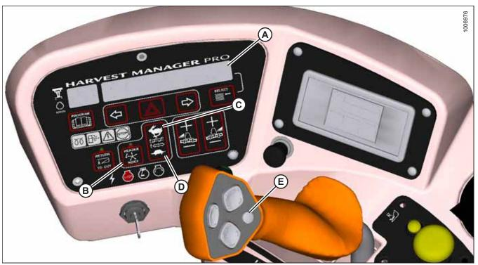
Figure 4.279: Operator Console
