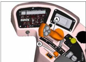
Figure 4.27: Operator Console
