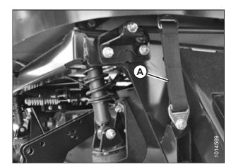
Figure 5.27: Cab Suspension
