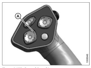
Figure 4.188: Ground Speed Lever
