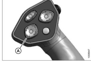
Figure 4.127: Ground Speed Lever
