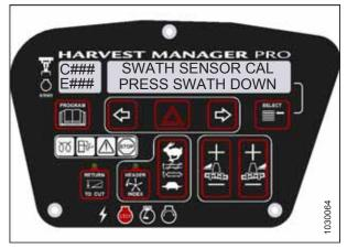
Figure 3.177: Swath Compressor Sensor Calibration
