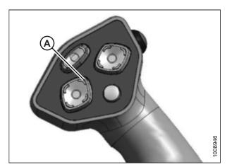
Figure 4.203: Ground Speed Lever
