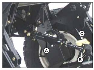
Figure 4.216: Hydraulic Center-Link
