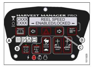
Figure 3.156: Reel Speed Control Lock
