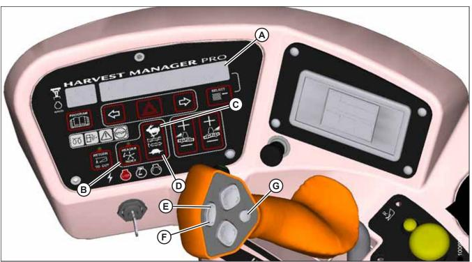
Figure 4.281: Operator Console
