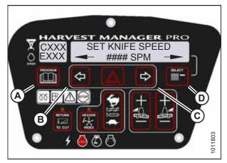
Figure 3.96: Knife Speed Setting
