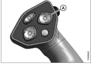
Figure 4.223: Ground Speed Lever
