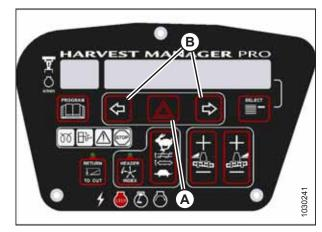
Figure 3.28: Turn Signal and Hazard Light Buttons on Cab Display Module
