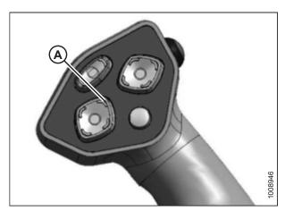
Figure 4.162: Ground Speed Lever
