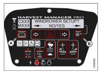
Figure 3.122: M155 CDM Programming Buttons Shown –M155*E4* M205 Similar
