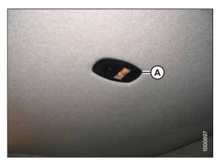
Figure 5.182: Ambient Light Fixture
