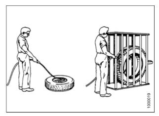
Figure 5.228: Safely Filling a Tire with Air
