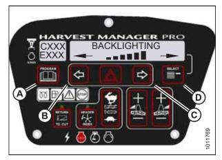
Figure 3.91: Display Backlighting Setting
