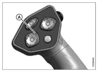
Figure 4.147: Ground Speed Lever
