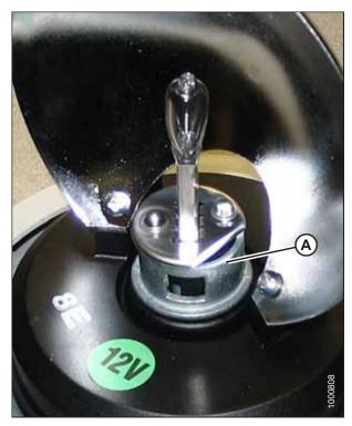
Figure 5.177: Beacon Lamp Assembly
