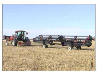
Figure 4.36: Towing a Header
