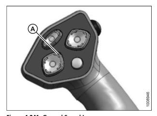
Figure 4.241: Ground Speed Lever
