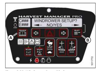
Figure 3.80: Windrower Setup Display
