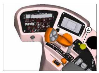
Figure 4.32: Header Drive Switch
