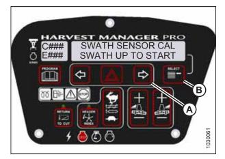
Figure 3.175: Swath Compressor Sensor Calibration
