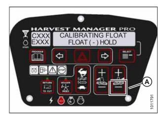
Figure 3.173: Negative Header Float Display
