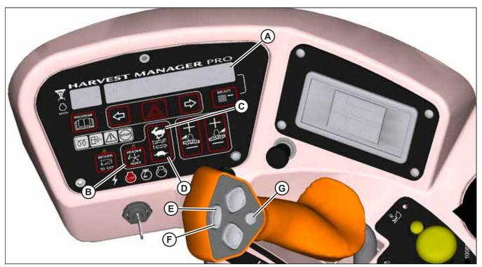
Figure 4.282: Operator's Console
