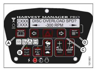
Figure 3.100: Disc Overload Speed
