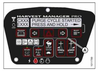
Figure 3.233: Hydraulic Purge Cycle
