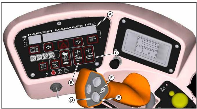
Figure 4.67: Cab Display Module (CDM)
