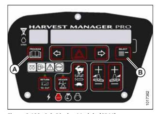
Figure 3.132: Cab Display Module (CDM)
