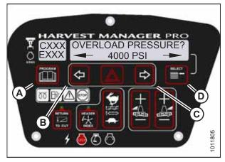
Figure 3.102: Hydraulic Overload Pressure
