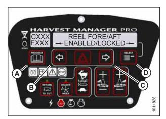
Figure 3.141: Reel Fore-Aft Control Lock
