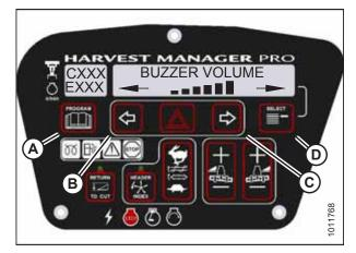
Figure 3.88: Buzzer Volume
