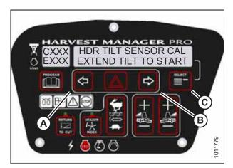
Figure 3.166: Header Tilt Calibration
