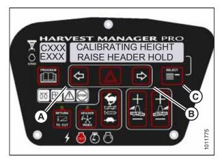
Figure 3.162: Header Height Calibration
