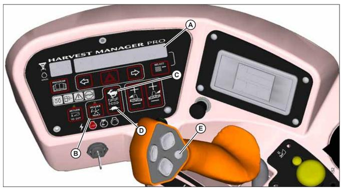
Figure 4.270: Operator Console
