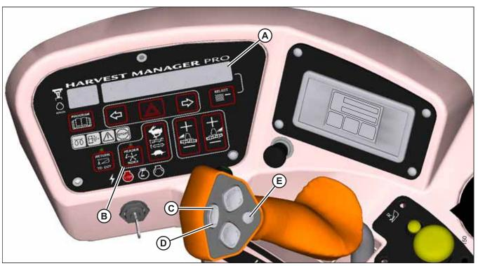
Figure 4.283: Operator Console
