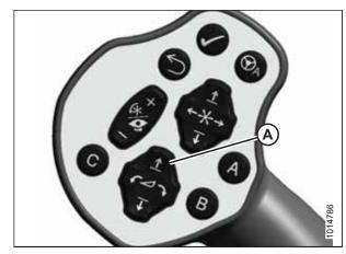
Figure 4.64: Ground Speed Lever
