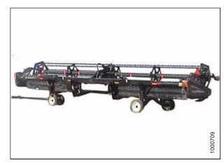
Figure 4.39: Header in Transport Mode
