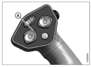
Figure 4.170: Ground Speed Lever
