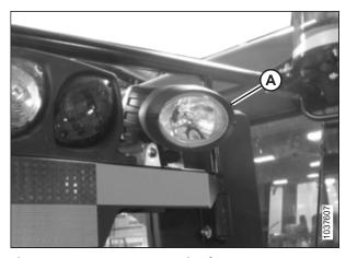
Figure 5.161: New HID Lamp in Place
