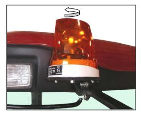
i. Turn the lens clockwise to lock it in place.
