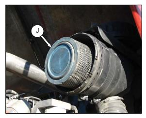
d. Pull out the primary filter element (J), and inspect as follows:
