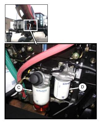
The M200 Windrower fuel system is equipped with primary (C) and secondary (D) filters.
