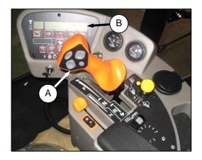
The GSL (A) contains switches for the following header functions that are most often adjusted while in operation to suit changing crop conditions.
