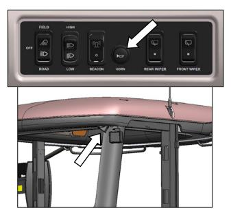
The horn is activated by pushing the button located on the panel in the headliner. The ignition switch must be on.
