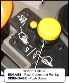
Engages and disengages header drive.
