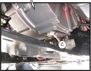
c. Remove drain plug (C), and allow the oil to completely finish draining.
