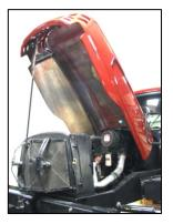
a. Shutdown the engine, and open engine compartment access hood to highest position.
