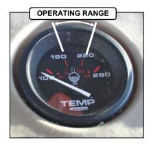
The normal engine operating temperature range is 180° - 225°F (82° - 107°C), and is indicated by a gauge on the Operator's console. If the temperature exceeds 230°F (110°C), an ongoing intermittent tone will be heard and the CDM will flash "ENGINE TEMP". Stop the engine immediately and determine cause. The tone will stop and the CDM will return to normal when the temperature drops below 225°F (107°C).
