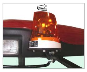
b. Turn lens counter clockwise to unlock lens from base, and remove lens.
