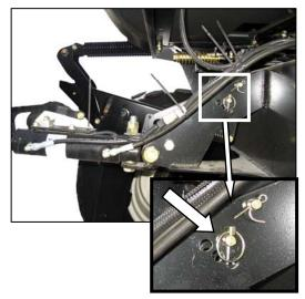
1. Relocate the pin at the frame linkage as required to position the hook over the header pin.
