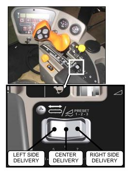
• Draper Header with Deck Shift Option Controls deck shifting for double windrowing options with a draper header.
