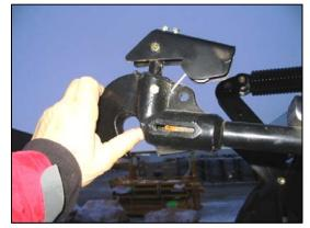
4. Push up on actuator rod (C) and pin should lift with the handle.
