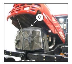
d. Turn the radiator cap (C) to the first notch to relieve pressure before removing cap completely. *(continued next page)*
