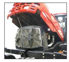
d. Open engine compartment hood to lowest position.
