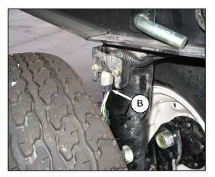
c. Disconnect wiring connector (B) at front wheel.
