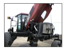
a. Shutdown the engine, and open engine compartment access hood to highest position.
