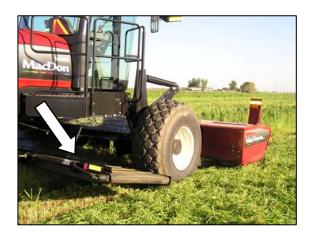
The double windrow attachment (DWA) allows the combining of two windrows of conditioned material close together to be picked up by a forage chopper. This unit may be mounted on the MacDon M150 and M200 Windrowers.
