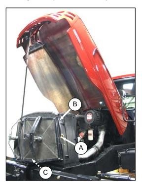
c. Push latch (A), and open screen assembly access door (B). Secure with rod (C) stored inside the screen door.
