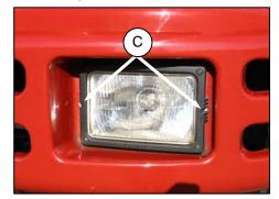
a. Remove the two screws (C), and remove headlight assembly from hood.
