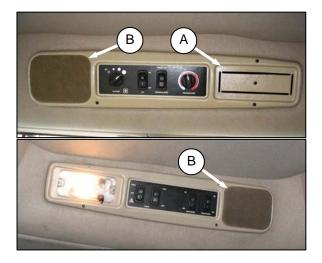
A radio is available as optional equipment from your MacDon Dealer, and a space (A) is provided in the cab headliner to accommodate the installation. Two pre-wired speakers (B) have been factory installed in the headliner.
