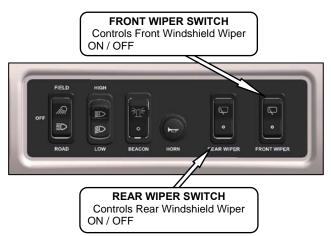
The windshield wiper controls are located in the cab headliner. The illustration above designates the controls as in the cab-forward mode.
