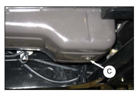
I. Install the oil pan drain plug (C).
