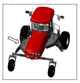
b. Move the left cab-forward platform to the open position for access to the coolant tank and radiator. Ensure the platform latch is engaged in open position.
