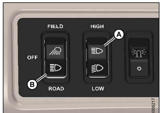
Figure 7.24: Exterior Light Switches
