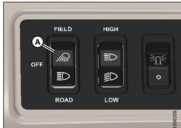
Figure 7.21: Exterior Light Switches
