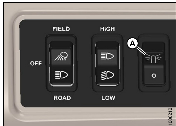
Figure 7.27: Exterior Light Switches
