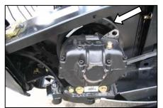
2. Check wobble box pulley speed with a handheld tachometer.
