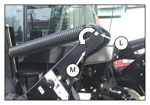
I. Remove pin (L) from storage position in linkage and insert in hole (M) to engage float springs. Secure with lynch pin.
