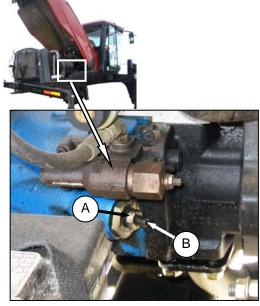
2. Loosen jam-nut (A).
