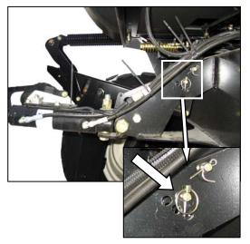
1. Re-locate the pin at the frame linkage as required to position the hook over the header pin.
