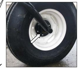
FORMED CASTER WHEEL BEARING 1 PLACE (BOTH WHEELS)
