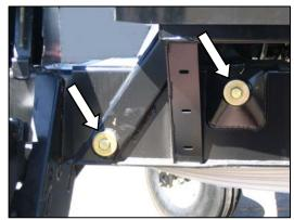
c. Remove two bolts, washers, and nuts from frame.
