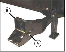
a. Remove hairpin from pin (A), and remove pin from left and right header boots (B) on header.
