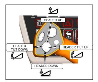
c. Start the engine and activate header down button on the GSL to fully retract header lift cylinders.
