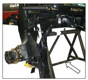
a. Support the front of the windrower off the ground with stand(s).
