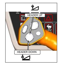
b. Start the engine and activate header down button on the GSL to fully retract header lift cylinders.
