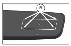
d. Remove the cut-out by cutting the tabs (B) in the panel. Remove sharp edges on panel.
