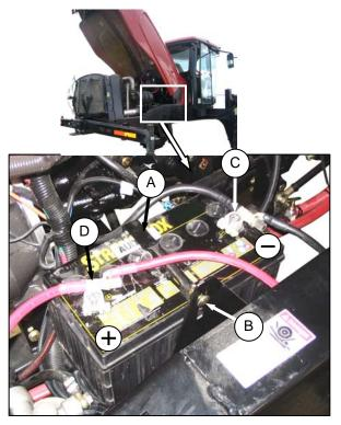
d. Install strap (A) with bolt (B) provided and tighten securely.
