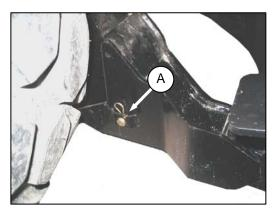
h. Install pin (A) through each boot and foot and secure with hairpin..
