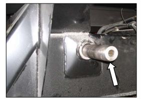
d. Tap out the two pins with a hammer.
