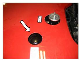
b. Turn filler cap counterclockwise to loosen bung, and remove dipstick.
