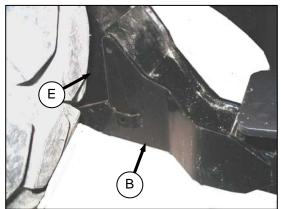
Slowly drive windrower forward so that feet (E) on windrower enter boots (B) on the header.
