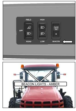
f. Switch on beacons (if installed) and check that they are functioning. The ignition switch must be at RUN but the engine does not need to be running.
