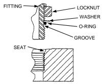
a. Inspect O-ring and seat for dirt or obvious defects.
