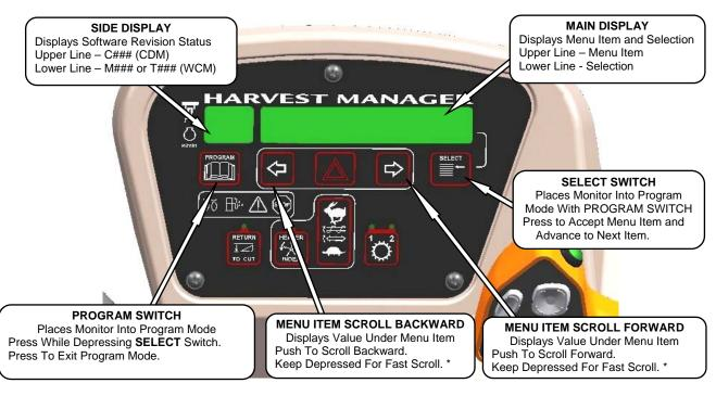
\* Fast scroll applies only when changing OVERLOAD SPEED (with expansion module), and TIRE SIZE.
