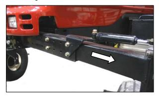
c. Slide extensions outboard equal amounts and align holes at desired location.
