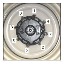
e. Install wheel nuts and tighten to 175-200 ft-lbf (237-271 N·m) using the tightening sequence as shown.
