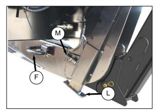
j. Install pin (F) through header leg, (engaging Ubracket in lift linkage) on both sides and secure with hairpin.
