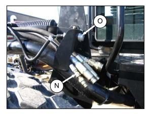
o. Connect header drive hydraulics (N) and electrical harness (O) to header. Refer to Auger Header Operator's Manual.
