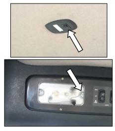
a. Switch lights on and off with switches on each light. Interior lights only work with road or field light switch on.
