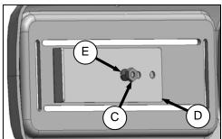
c. Remove screw and nut (C) to remove support (D) from panel. Retain metric nut (E) and lockwasher.
