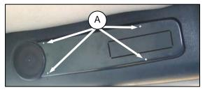
b. Remove radio panel by removing four screws (A).
