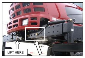
b. Remove six bolts (four on backside, two on underside) and washers from left and right side of walking beam.
