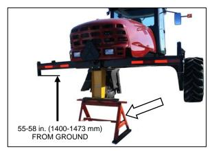
a. Support rear of windrower with jack stands under the rear frame or with a support under the shipping stand. Distance between walking beam and ground should be 55-58 in. (1400-1473 mm).
