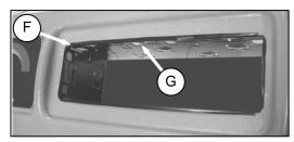
e. Locate receptacle (F) (supplied with radio) in opening and secure by bending tabs (G) on receptacle against panel.
