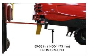
a. Support rear of windrower with a forklift or equivalent. Distance between walking beam and ground should be 55-58 in. (1400-1473 mm).
