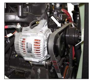
Tension on fan belt should be such that a force of 22 lbf (100 N) deflects belt 5/16 to 1/2 in. (8 to 12 mm) at mid-span.
