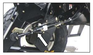
The hydraulic center link is supplied in a separate kit that is included with the shipment. Refer to installation instructions in the kit.
