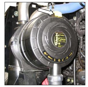
a. Check that air cleaner cap is firmly attached and that all clamps on air cleaner are secure.
