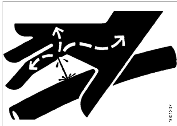
Figure 1.12: Hydraulic Pressure Hazard
